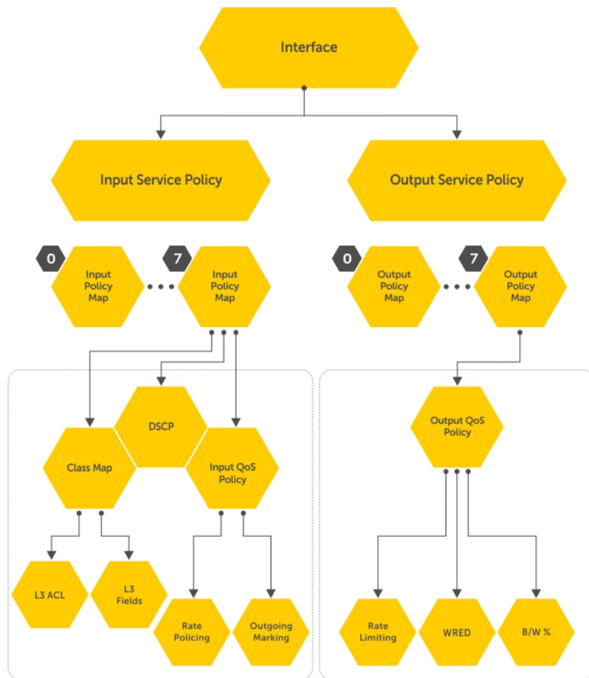
Figure 103. Constructing Policy-Based QoS Configurations
