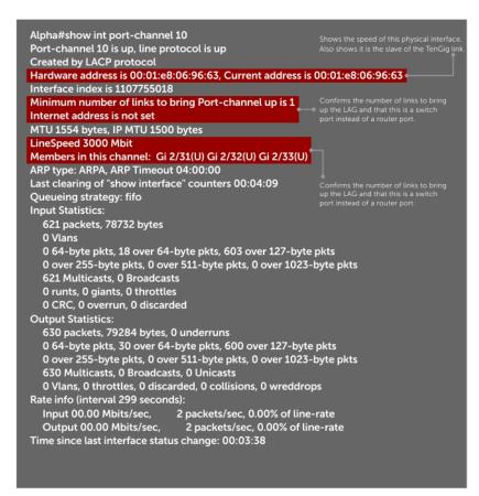
Figure 69. Inspecting Configuration of LAG 10 on ALPHA
