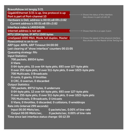
Figure 71. Inspecting a LAG Port on BRAVO Using the show interface Command
