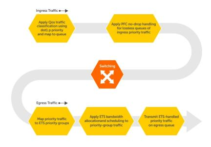
Figure 31. DCB PFC and ETS Traffic Handling
