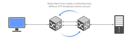
Use backup interfaces to create redundant links in networks without STP
