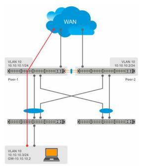
Figure 147. Packets with peer routing enabled
