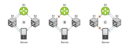
A. Switches 1 and 2 have upstream and downstream connections to Router1 and Server via primary Links.
