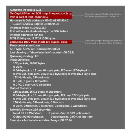
Figure 68. Inspecting the LAG Configuration
