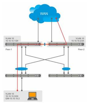
Figure 146. Packets without peer routing enabled
