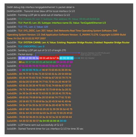
Figure 85. The debug Ildp detail Command — LLDPDU Packet Dissection
