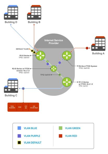
Figure 121. Single and Double-Tag First-byte TPID Match
