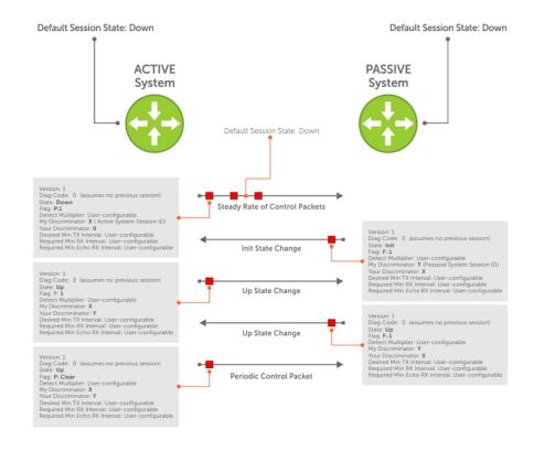
Figure 10. BFD Three-Way Handshake State Changes
