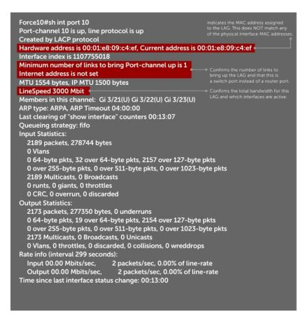
Figure 72. Inspecting LAG 10 Using the show interfaces port-channel Command
