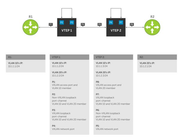
In this RIOT scheme, whenever R1 tries to reach R2, the packet gets to P1 on VTEP 1 with VLAN 10 and gets routed out of P2 on VLAN 20. VTEP 1 sends an ARP request for R2 (10.1.2.1) through P2. This request gets VXLAN encapsulated at P3 and is sent out of P4. Eventually, the native ARP request reaches R2.
