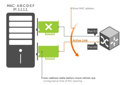
Figure 75. Configuring the mac-address-table station-move refresh-arp Command
