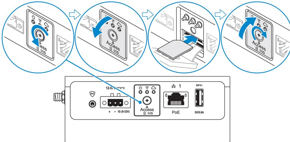
3. Replace the screw, and close the micro-SIM card access door.
