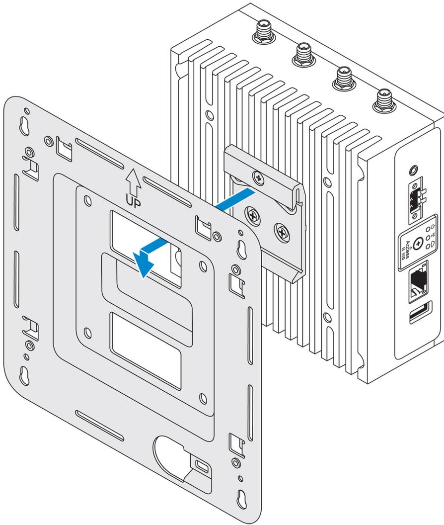
9. Push the Edge Gateway towards the DIN-rail to secure it on the standard-mount bracket.
