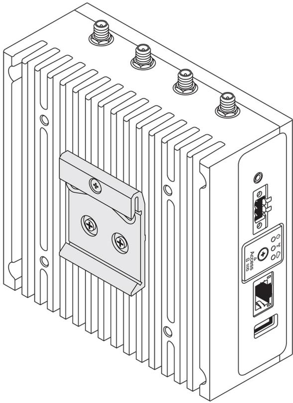
4. Place the Edge Gateway on the DIN rail at an angle, and then pull the Edge Gateway down to compress the springs at the top of the DIN-rail mounting bracket.
