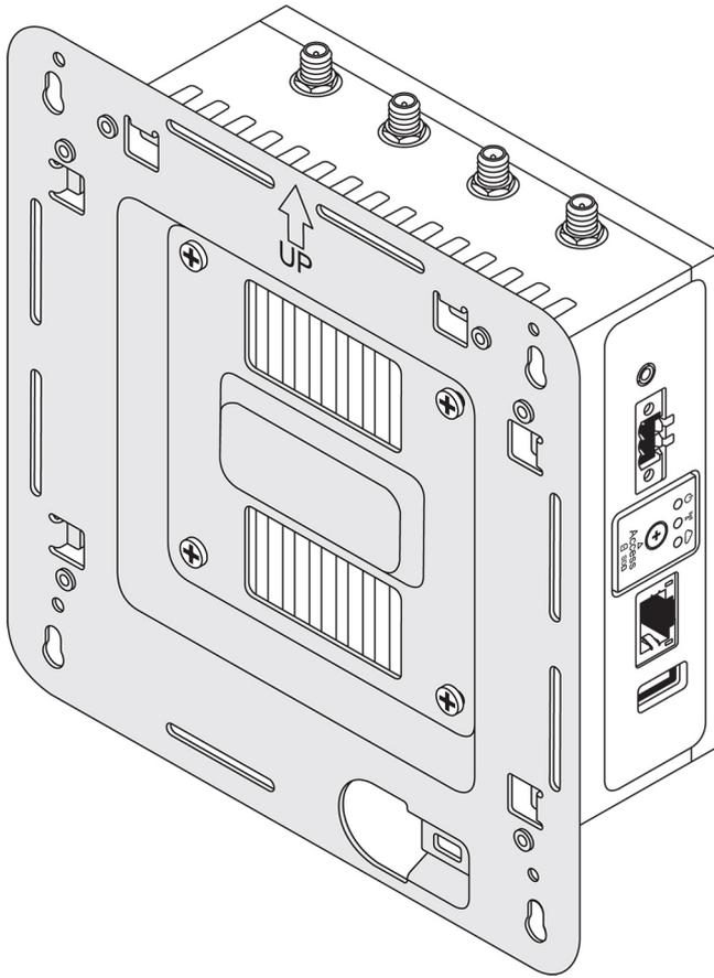
3. Place the standard-mount bracket on the wall, and using the holes above the screw holes on the bracket, mark the positions to drill the four holes.
