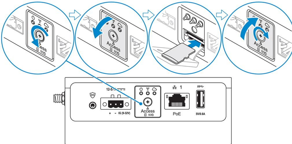
**NOTE:** Remove the SD card slot filler before inserting a micro-SD card.
