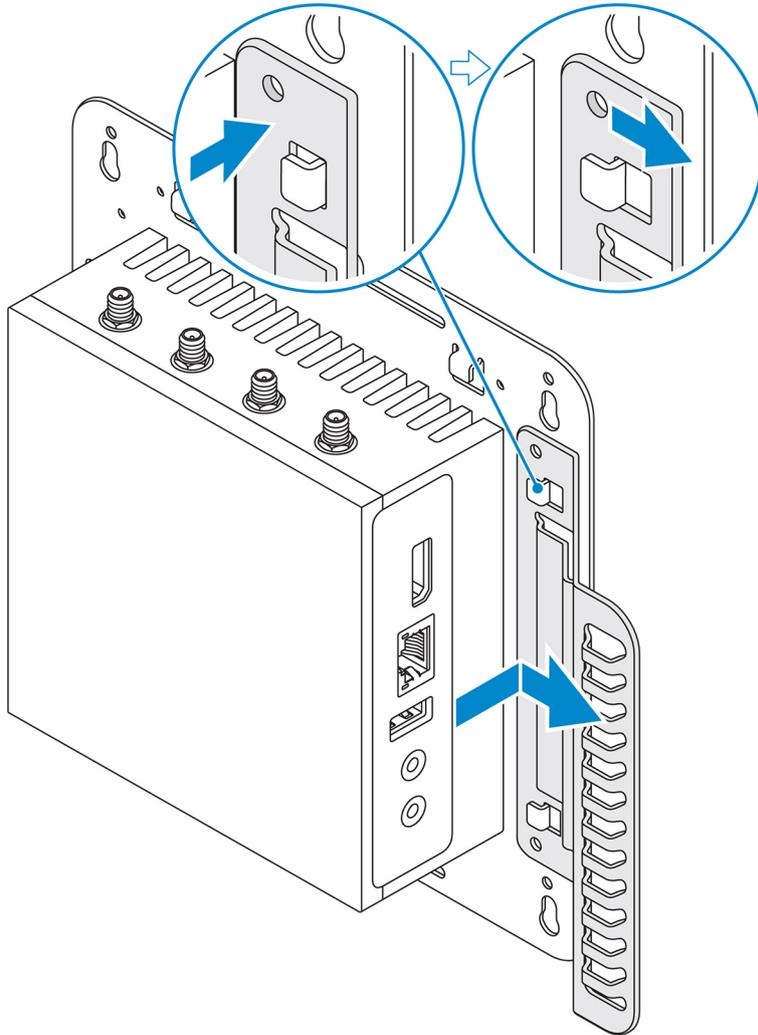
3. Align the screw holes on the cable control bar with the screw holes on the mounting bracket.
