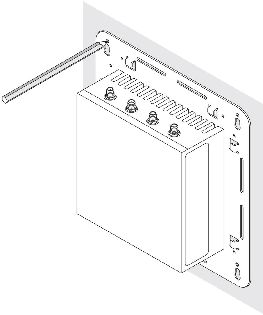
4. Drill four holes in the wall as marked.
