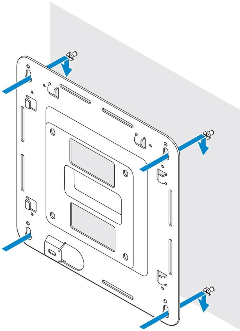
5. Tighten the screws to secure the assembly to the wall.
