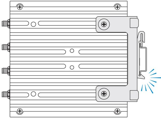
6. Secure the Edge Gateway on the DIN rail.
