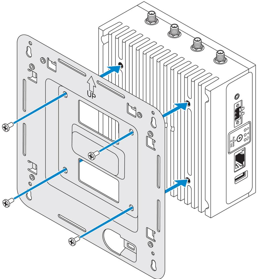
2. Place the Edge Gateway against the wall, and align the holes in the standard-mount bracket with the holes on the wall. Screw holes on the bracket have a diameter of 3 mm (0.12 in).
