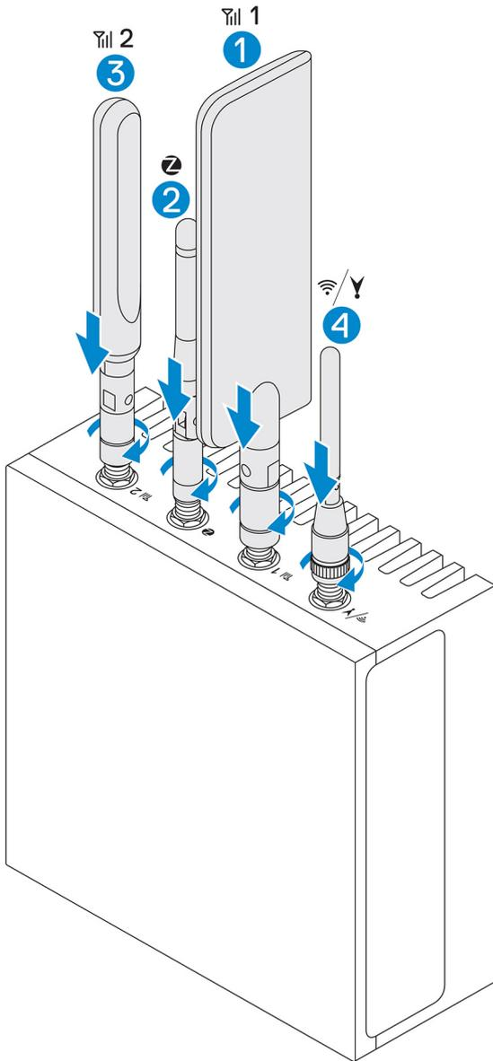
4. Secure the antenna by tightening the rotating head of the connector until it firmly holds the antenna in the preferred position (upright or straight).
