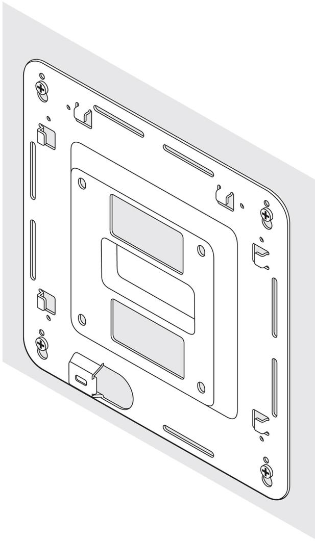
6. Align the screw holes on the DIN-rail bracket with the screw holes at the back of the Edge Gateway.
