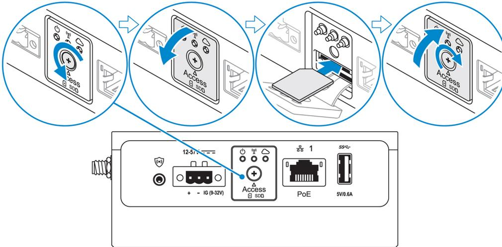
8. Insert a micro-SD card into the bottom micro-SD card slot.
