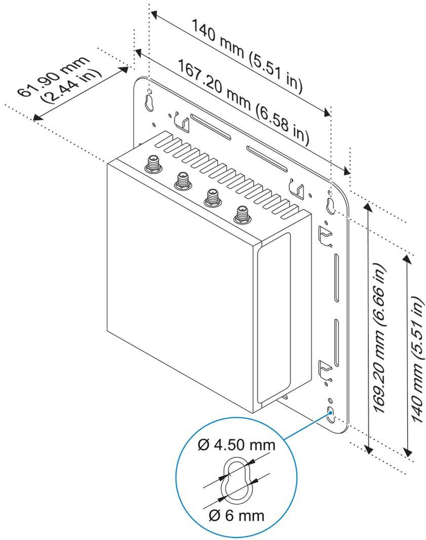
**NOTE:** The mounting brackets are shipped with only those screws that are required for securing the mounting brackets to the Edge Gateway.
