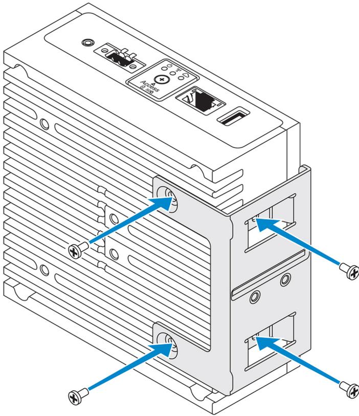
3. Align the screw holes on the DIN-rail mount bracket with the screw holes on the perpendicular-mount bracket, and tighten the two screws.
