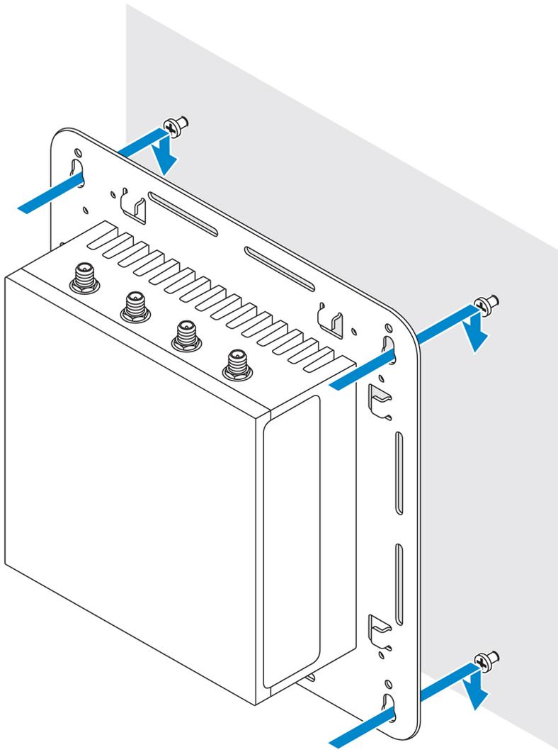
**7.** Tighten the screws to secure the assembly to the wall.
