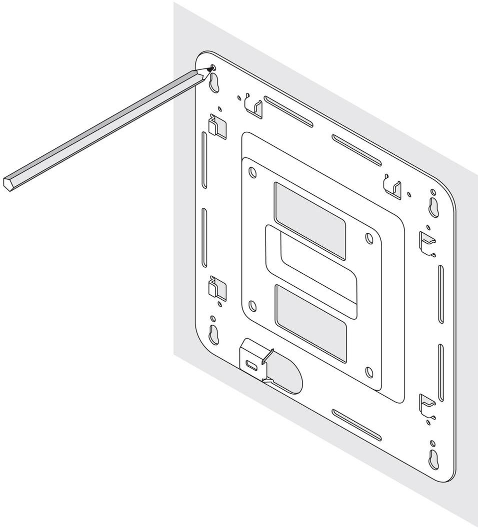
2. Drill four holes in the wall as marked.
