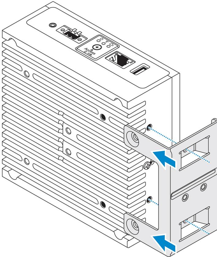
2. Tighten the four M4x7 screws to secure the Edge Gateway to the perpendicular-mount bracket.
