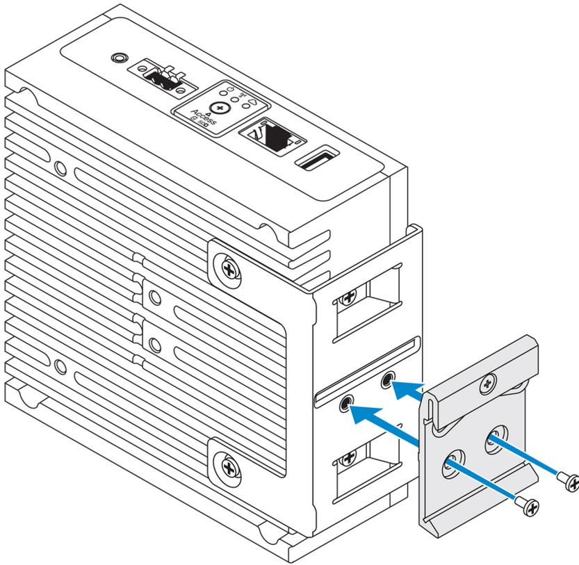
4. Place the Edge Gateway on the DIN rail at an angle and push the Edge Gateway down to compress the springs on the DIN-rail mount brackets.
