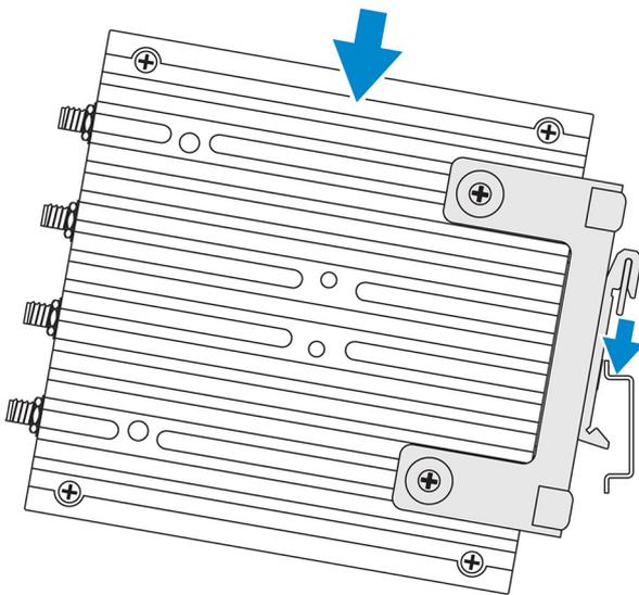
5. Push the Edge Gateway towards the DIN-rail to secure the lower clip of the bracket onto the DIN rail.
