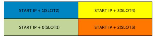
The following figure shows the QuickDeploy IP addresses assignment to the servers when there are two full-height blades in VRTX chassis:
