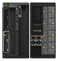
To view the chassis health, click **Chassis Overview**. The system displays the overall health status of the chassis, active and standby CMCs, server modules, IO Module (IOM), fans, blowers, power supply units (PSUs), LCD assembly, storage controller, and PCle devices. Detailed information about each component is displayed when you click that component. In addition, the latest events in the CMC Hardware Log are also displayed. For more information, see the *Online Help*.
