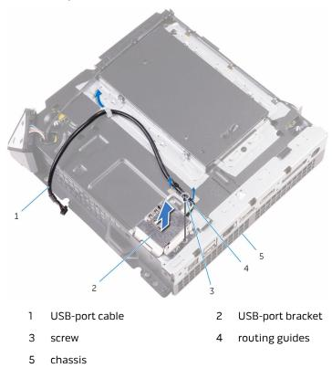
Remove the screw that secures the USB port to the chassis.
