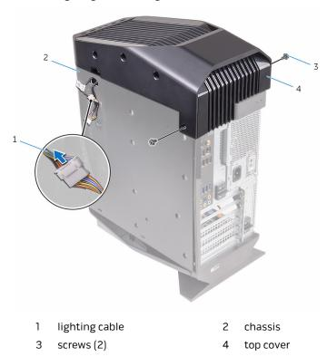
Starting from the rear, release the tabs on the top cover from the slots on the chassis.
