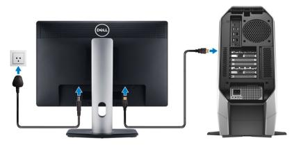
NOTE: The DisplayPort on the back panel of your computer is covered. Connect the display to the discrete graphics card of your computer.
