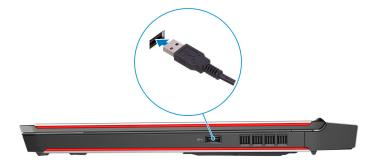
3. Connect a USB Type-C to Type-A dongle to the Thunderbolt 3 (USB Type-C) port on the back of your computer.
