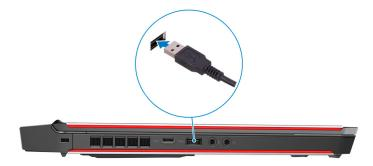
5. Connect a USB Type-C to Type-A dongle to the USB 3.1 Gen 2 (Type-C) port at the left side of your computer.
