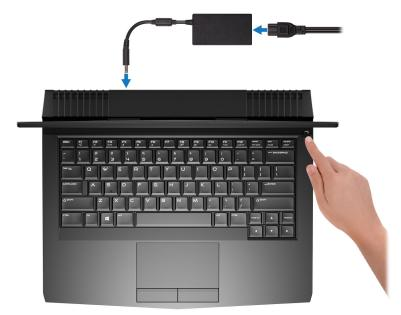
Connect the power adapter and press the power button.
