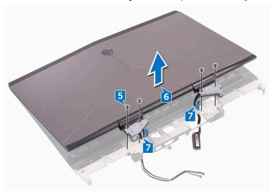
8 Place the display assembly on a clean, flat surface.
