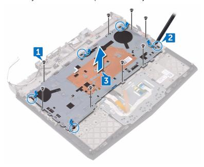
4 Lift the keyboard at an angle and remove it from the tabs on the palm-rest assembly.
