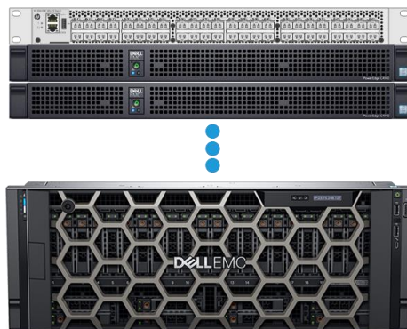
Figure 3: SQream DB on Dell PowerEdge R940xa reference architecture featuring additional PowerEdge C4140 compute nodes for scale-out
