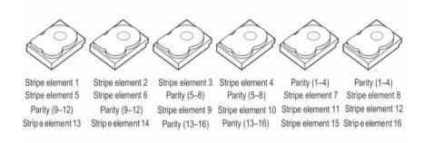
Figure 9. Example of Dual Distributed Parity (RAID 6)
