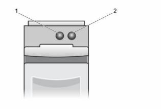
Figure 5. Disk Carrier LED Indicators
