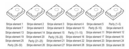
Figure 8. Example of Distributed Parity (RAID 5)
