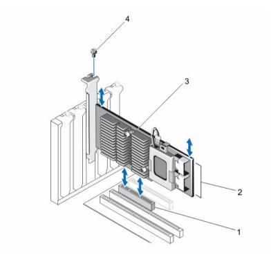
Figure 1. Removing and Installing the PERC Adapter
