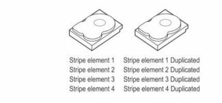
Figure 7. Example of Disk Mirroring (RAID 1)
