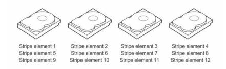
Figure 6. Example of Disk Striping (RAID 0)
