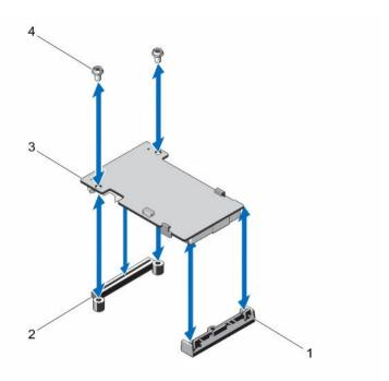
Figure 2. Removing and Installing the PERC Mini Blade Controller
