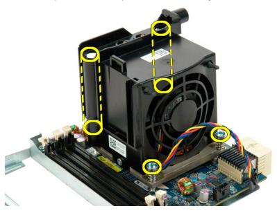
13. Remove the dual processor heat sink fan assembly from the dual processor riser board.
