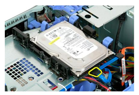
6. Lift the two blue hard drive release tabs.
