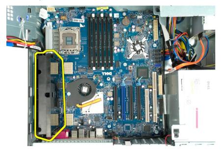
17. Remove the eight screws that secure the system board to the computer chassis.
