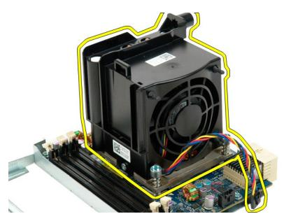
14. Release the dual processor cover by pressing down and out on the release arm.
