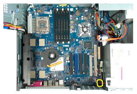
11. Disconnect the I/O data cable from the system board.
