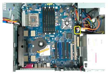
13. Disconnect the power supply cable from the system board.
