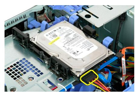
4. Disconnect the power cable from the first hard drive.
