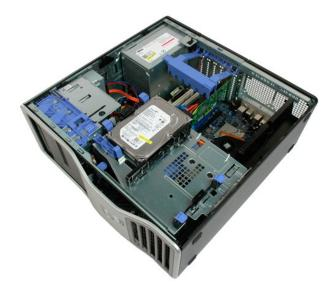
3. Press the hard drive release lever toward the bottom of the computer.
