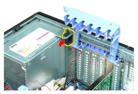
${\bf 6.} \quad {\bf Remove \ the \ intrusion \ switch \ from \ the \ computer.}$
