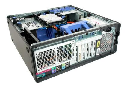
3. Remove the four screws securing the power supply on the outside of the computer.
