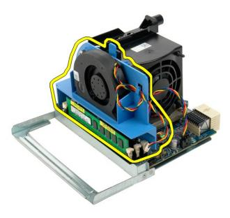
8. While pressing on the blue release tab, remove the dual processor fan assembly from the dual processor assembly.
