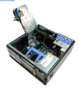
5. Disconnect the two fan cables from the system board.
