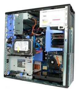
3. Disconnect the power cable from the back of the optical drive.
