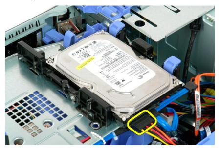
5. Disconnect the data cable from the first hard drive.
