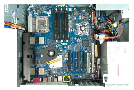
10. Disconnect the intrusion switch cable from the system board.
