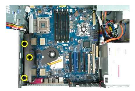
16. Remove the dual processor riser.
