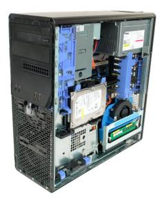
3. Pull down on the dual processor riser release lever.
