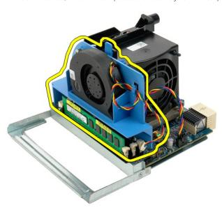
9. Gently press down on the memory module release tabs to release the first dual processor memory module from the connector.
