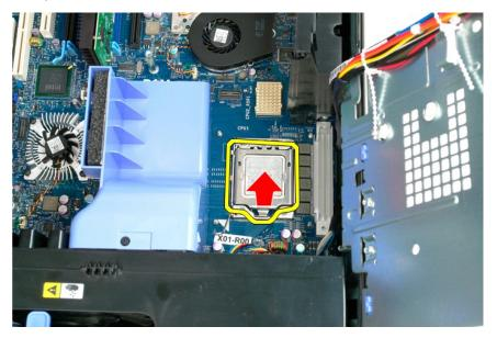
8. Lift the processor straight up and remove it from the computer.
