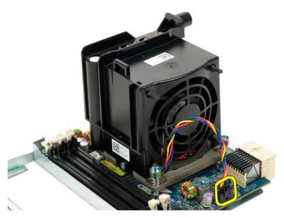
12. Loosen the four captive screws on the dual processor heat sink/fan assembly.
