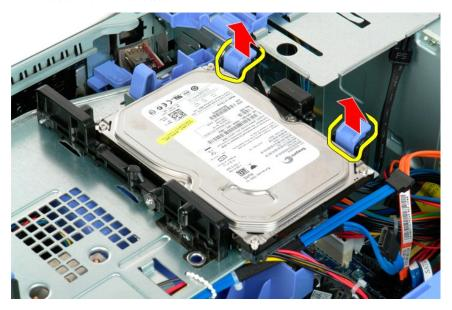
7. Remove the first hard drive assembly from the computer. Repeat these steps for any other installed hard drives.
