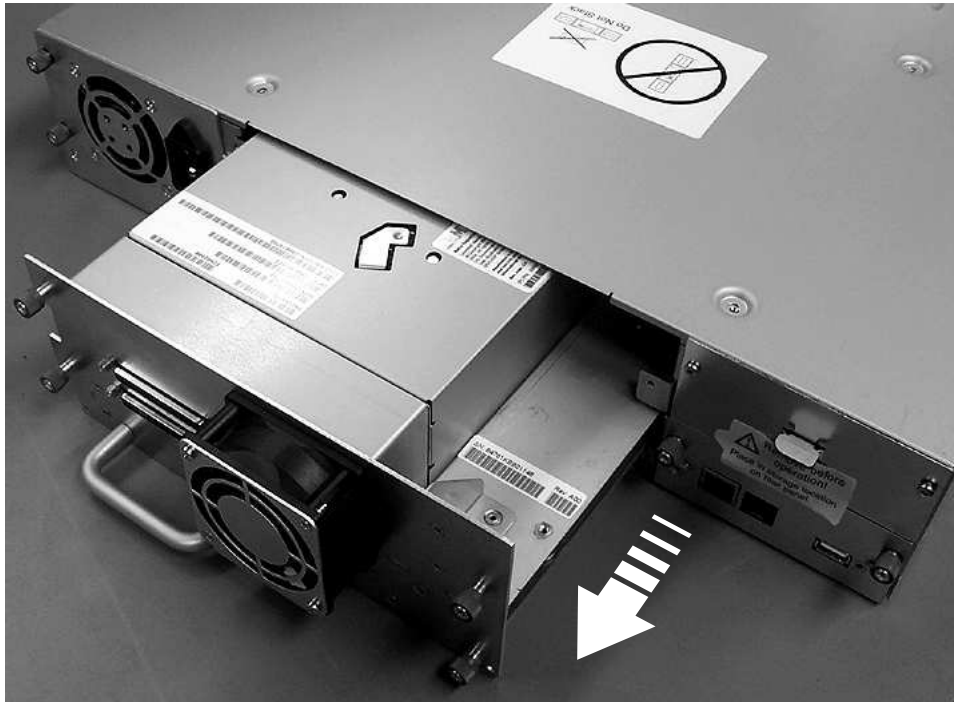
Figure 151. Removing a drive sled from the library (drive sled without ESD springs shown)
