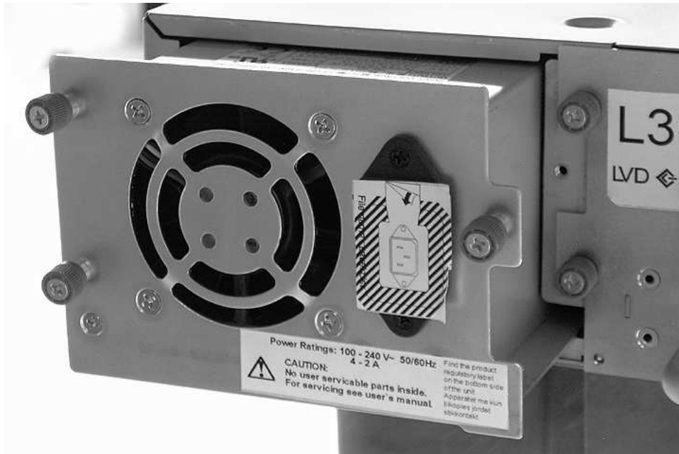
Figure 153. A power supply being removed from a library
