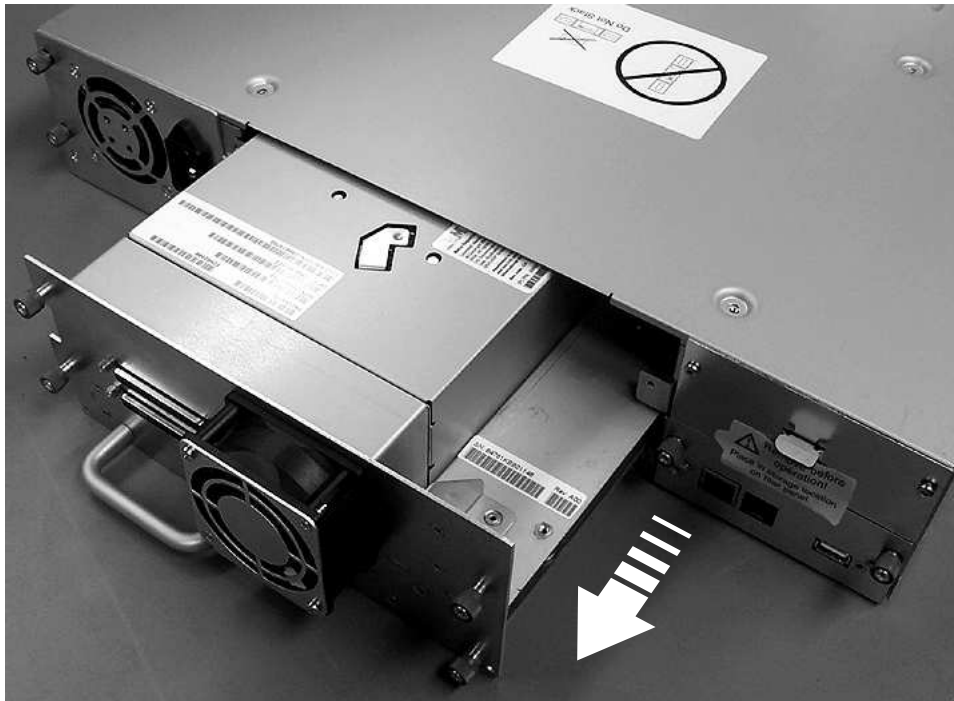
Figure 142. Pulling the drive sled out of the library (drive sled without ESD springs shown)
