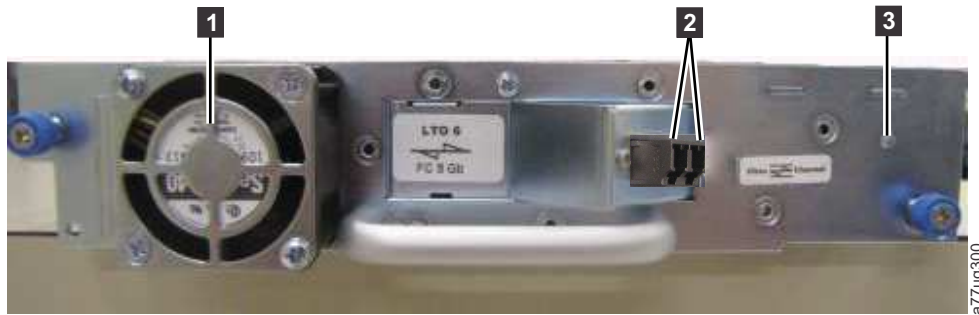
Figure 3. Rear panel (drive sled only) of a half height Fibre Channel drive
