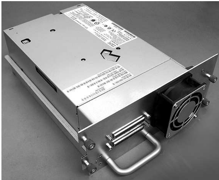
Figure 6. Library drive sled without ESD springs (SCSI sled shown)
