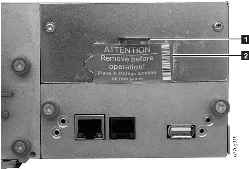
Figure 150. Library shipping lock and label storage location on the rear panel of the library
