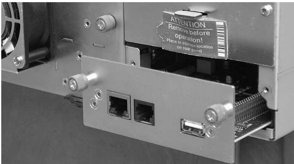
Figure 154. Removing a Library Controller Card from the library
