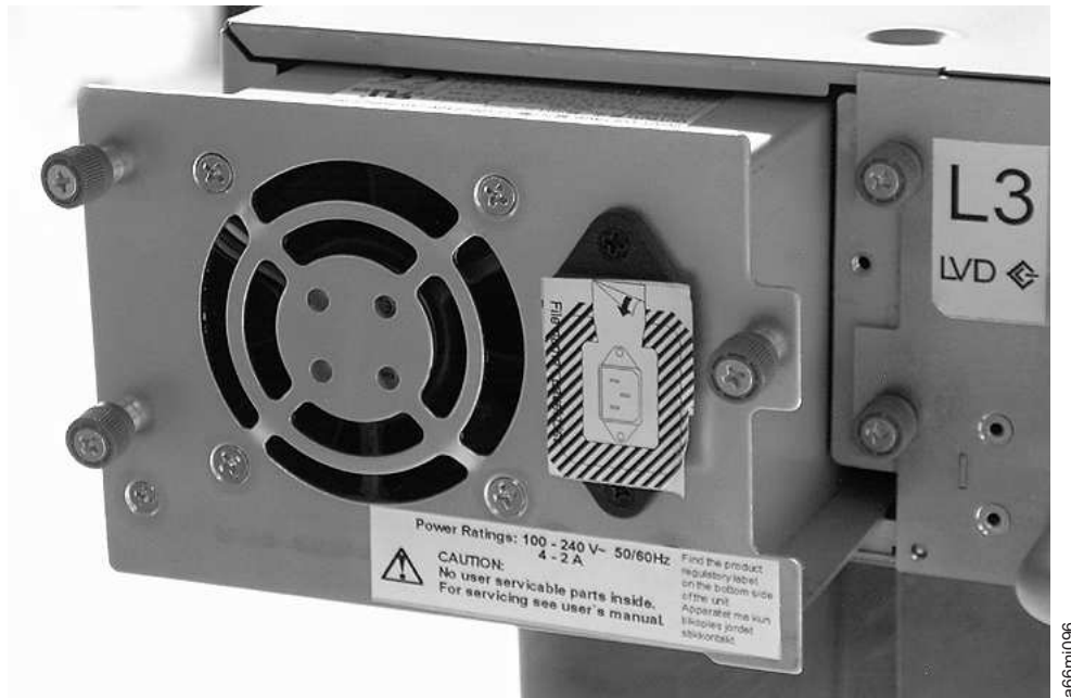
Figure 145. A power supply being removed from a 2U library
