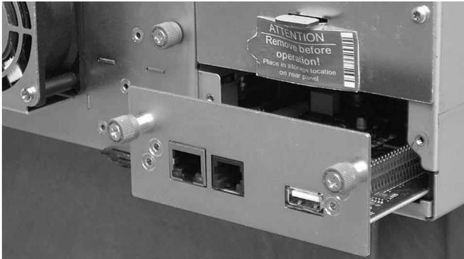
Figure 146. A Library Controller Card being removed from the library
