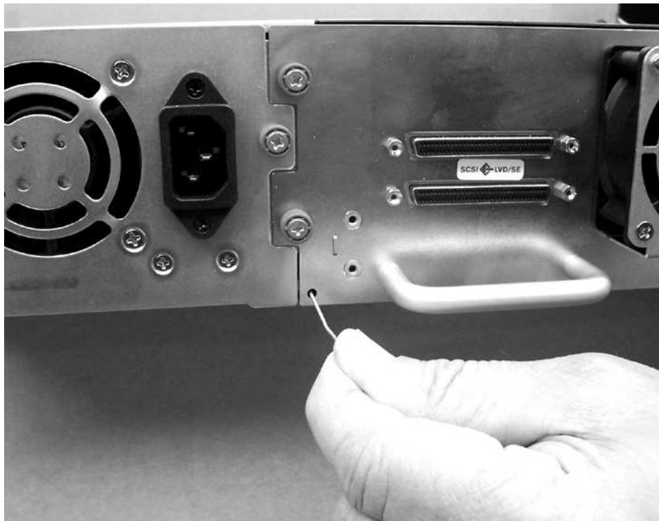
Figure 156. Access hole for the left magazine (facing rear of library)
