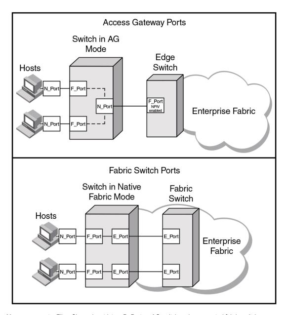
You can convert a Fibre Channel port into a D\_Port on AG switch and a connected fabric switch, another AG switch (cascaded configuration), or an HBA to test the link between the ports. When you configure the ports on each end of the link as D\_Ports, diagnostic tests automatically initiate on the link when the D\_Ports go online. Results can be viewed using Fabric OS commands, such as
