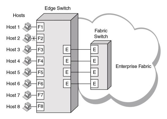
FIGURE 2 Switch function in Access Gateway mode
