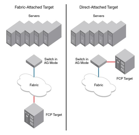
Although target devices can be connected directly to AG ports, it is recommended that the switch operating in AG mode be connected to the core fabric.
