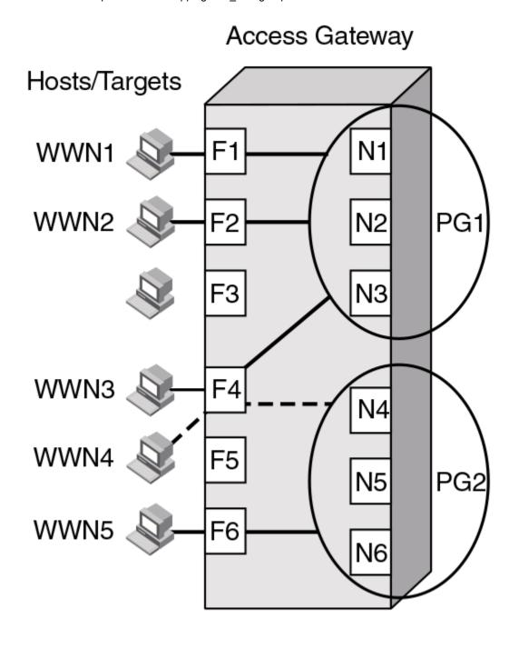
The figure below shows an example of device mapping to specific N\_Ports. Note that you can map one or multiple WWNs to one N\_Port to allow multiple devices to log in through one N\_Port.
