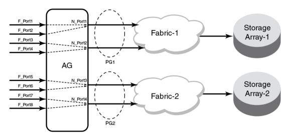
When a dual redundant fabric configuration is used, F\_Ports connected to a switch in AG mode can access the same target devices from both of the fabrics. In this case, you must group the N\_Ports
