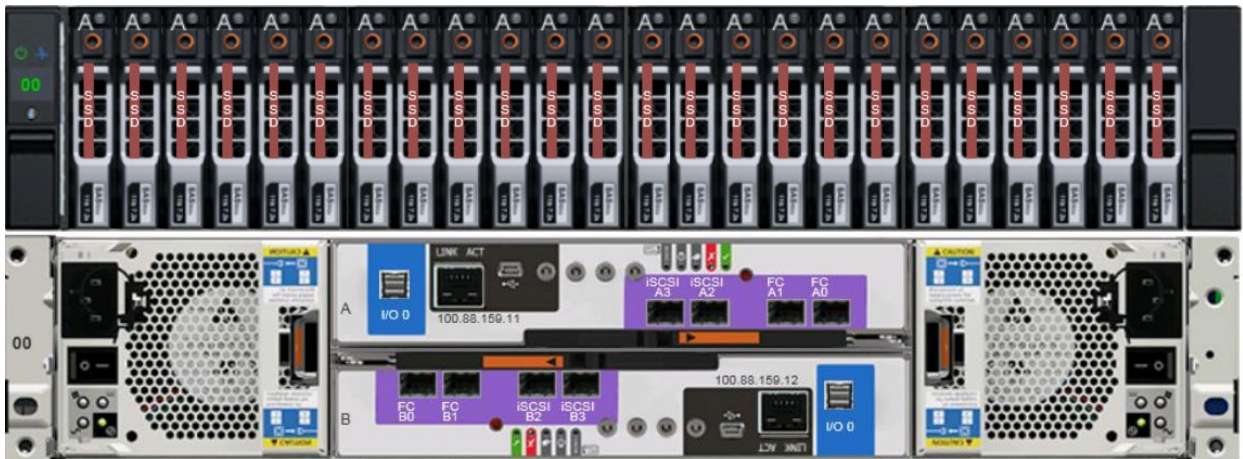
Figure 1: Front and rear view of the Dell EMC PowerVault ME4024 array, configured with 24 SSD drives and dual controllers
