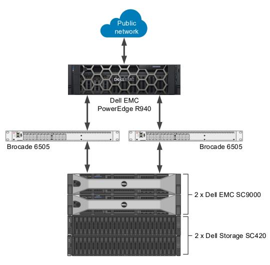
Figure 1 Single-server reference architecture
