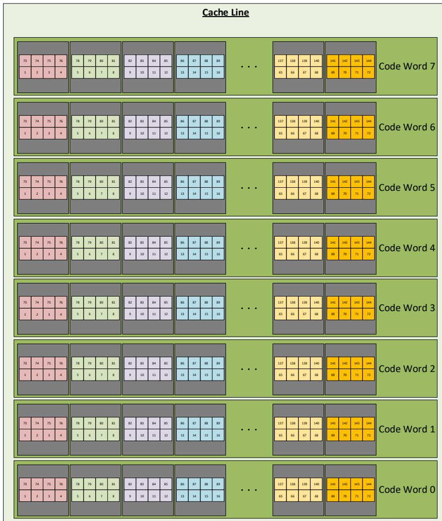
Figure 1 - Example Implementation of 8-Bit Symbol Size Advanced ECC
