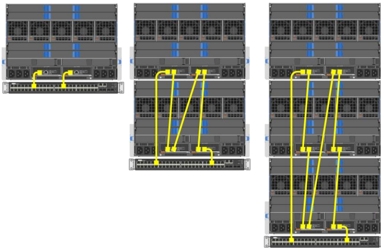
Figure 1 MCM group cabling one, two, or three chassis
