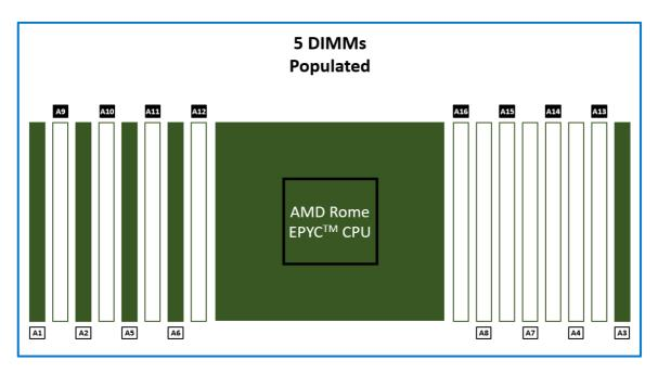
Figure 15: Five DIMMs are populated in an unbalanced configuration
