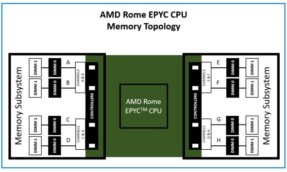
Figure 1: CPU-to-memory subsystem connectivity for Rome processors
