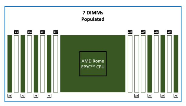
Figure 17: Seven DIMMs are populated in an unbalanced configuration
