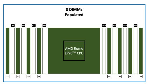
Figure 8: Eight DIMMs are populated in a balanced configuration, producing the highest memory bandwidth while at a lower capacity than sixteen
