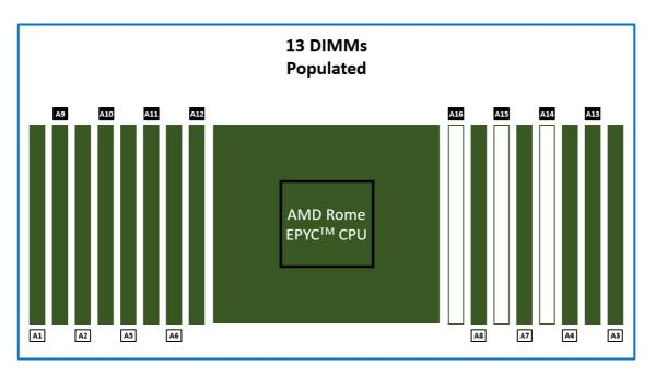
Figure 21: Thirteen DIMMs are populated in an unbalanced configuration
