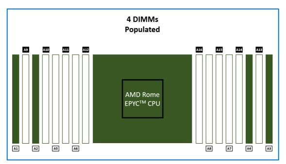
Figure 10: Four DIMMs are populated in a near balanced configuration
