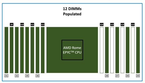
Figure 11: Twelve DIMMs are populated in a near balanced configuration
