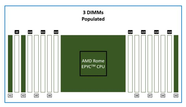
Figure 14: Three DIMMs are populated in an unbalanced configuration
