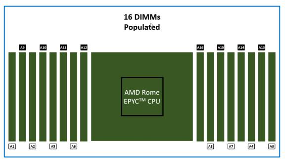
Figure 9: Sixteen DIMMs are populated in a balanced configuration, producing the highest memory capacity while at a lower bandwidth than eight
