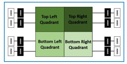
Figure 2: Quadrant layout of Rome processors
