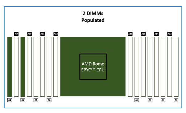
Figure 13: Two DIMMs are populated in an unbalanced configuration
