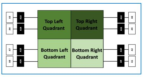
Figure 6: DIMM population order, starting with A1 and ending with A16
