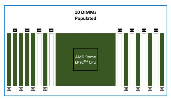
Figure 19: Ten DIMMs are populated in a near balanced configuration
