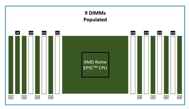
Figure 18: Nine DIMMs are populated in an unbalanced configuration
