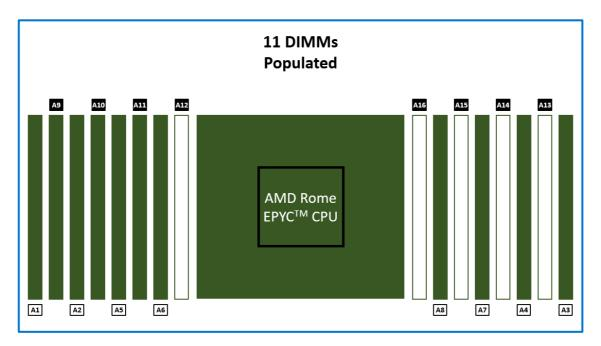
Figure 20: Eleven DIMMs are populated in an unbalanced configuration
