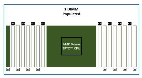
Figure 12: One DIMM is populated in an unbalanced configuration
