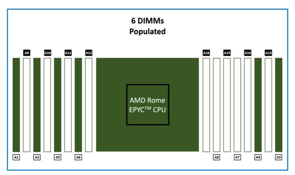
Figure 16: Six DIMMs are populated in a near balanced configuration
