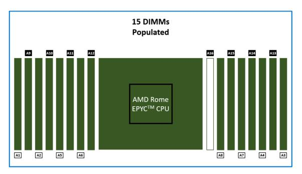
Figure 23: Fifteen DIMMs are populated in an unbalanced configuration
