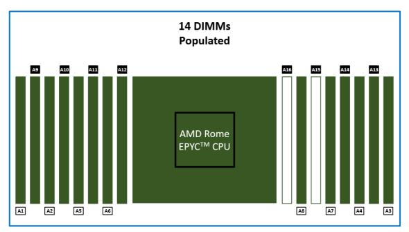
Figure 22: Fourteen DIMMs are populated in a near balanced configuration
