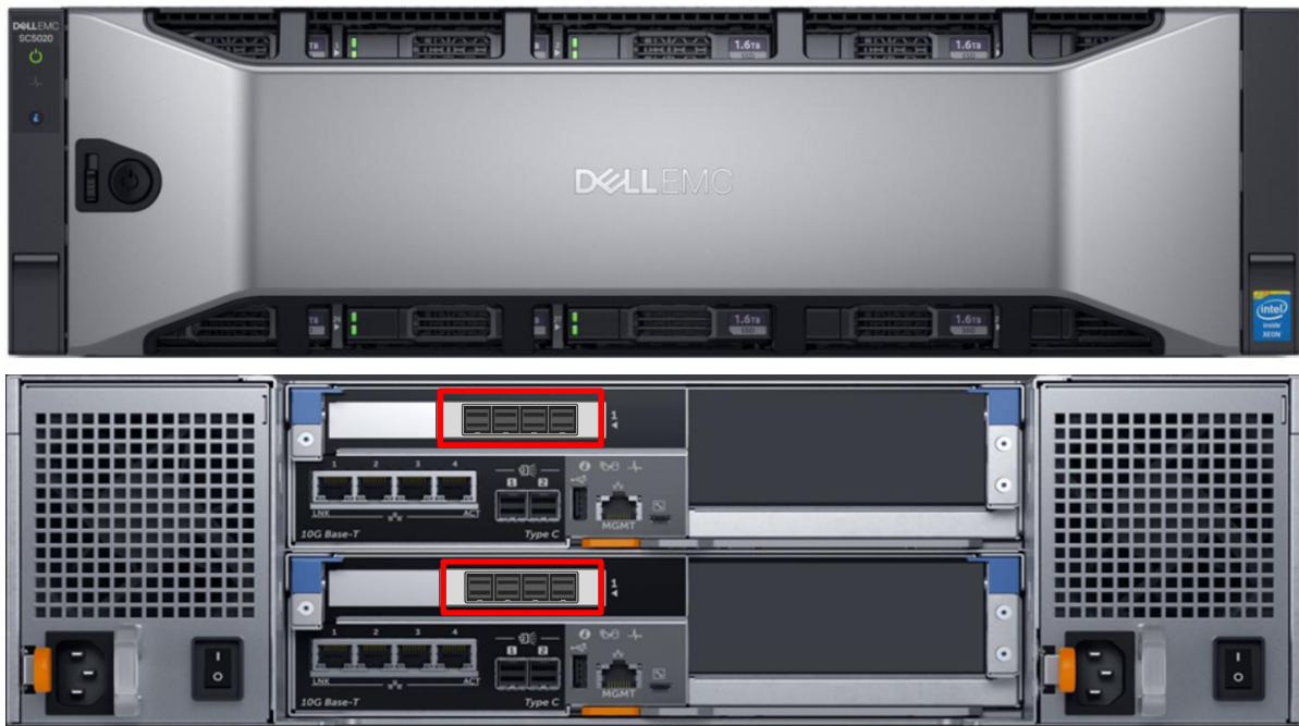
Figure 2 Front and rear views of an SCv3000/SC5020 array with SAS FE ports
