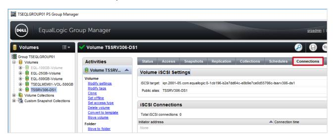
**Note:** It is strongly recommended to take a snapshot of the VMware volume hosted on the PS Series array before proceeding in online or offline mode. In the unlikely event of a failure during the import, a snapshot ensures volume integrity in the case of a restore.
