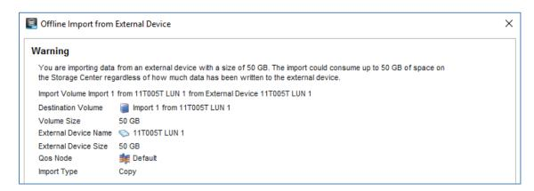
8. While the import process is running, monitor the progress in the volume details window. Click the **refresh** icon to update the progress.
