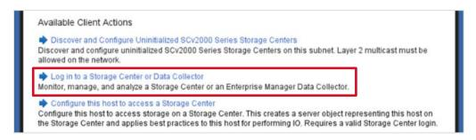
**Note:** The Dell Storage Client can connect to a Dell Storage Manager Data Collector or connect directly to an SC Series array. Both options are supported with the Thin Import process. The instructions in this section focus only on connecting directly to an SC Series array. Thin Import requires Dell Storage Client/Dell Storage Manager Data Collector version 2015 R2.
