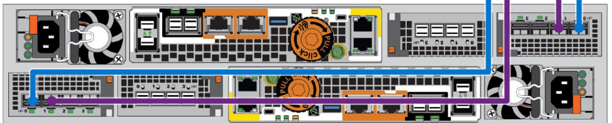
Figure 2 Dell EMC Unity cabling diagram
