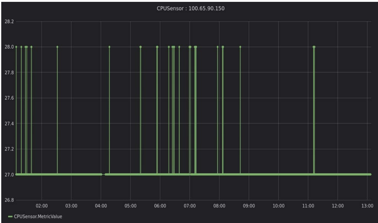
Figure 11 A time lapse Grafana plot of Exhaust Temperature from CPUSensor report
