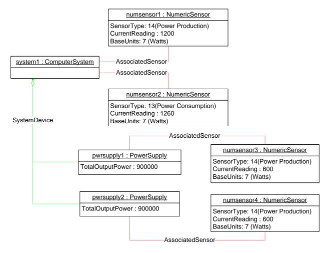
Figure 5 – Power Supply Profile: Power Sensors
