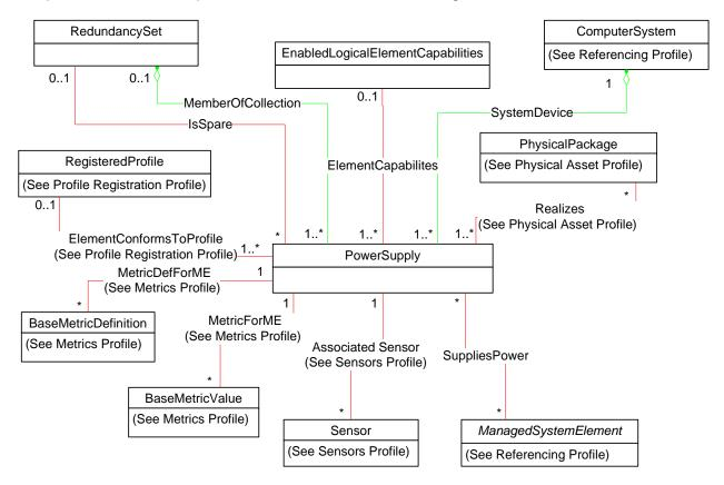
Figure 1 – Power Supply Profile: Class Diagram
