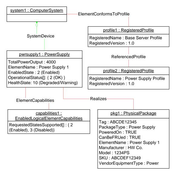
Figure 2 – Power Supply Profile: Object Diagram
