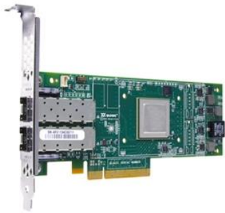
Figure 8 QLogic 32Gb FC PCIe card with two host server ports (HBAs)
