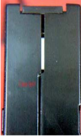
Figure 5 Split Seam on LTO Tape
