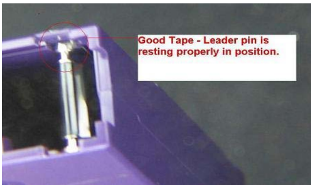
Figure 6 Media Inspection - Good Tape
