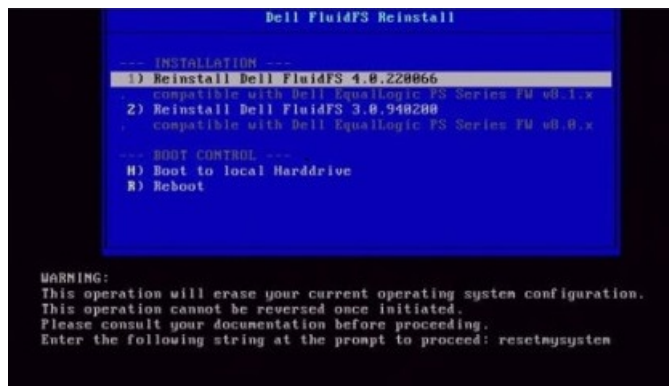
Figure 14. Dell FluidFS Reinstallation Menu
