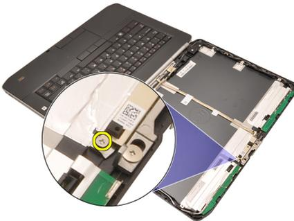
7. Lift and remove the camera module.
