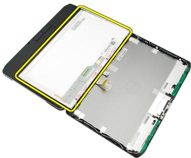
7. Remove the screws that secure the display brackets to the display panel and remove the brackets.
