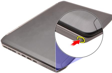
3. Press in on the PC latch to release the PC card.
