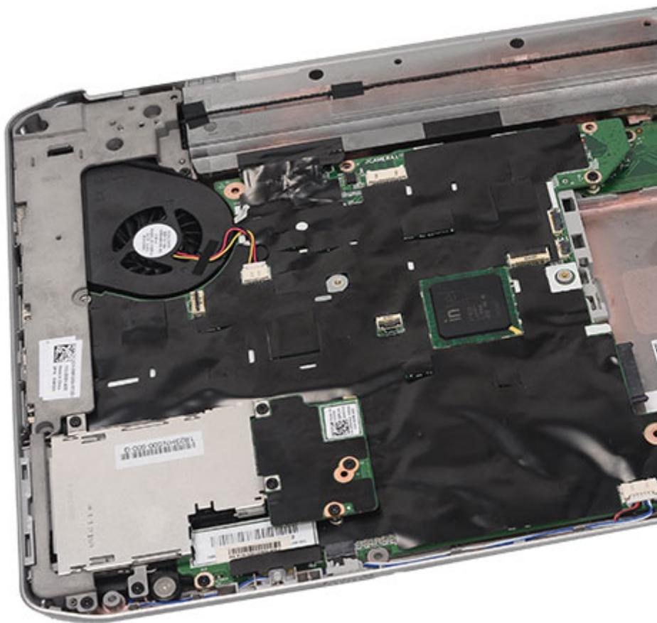
13. Lift the modem card, to disengage from the connector on the back of the card.
