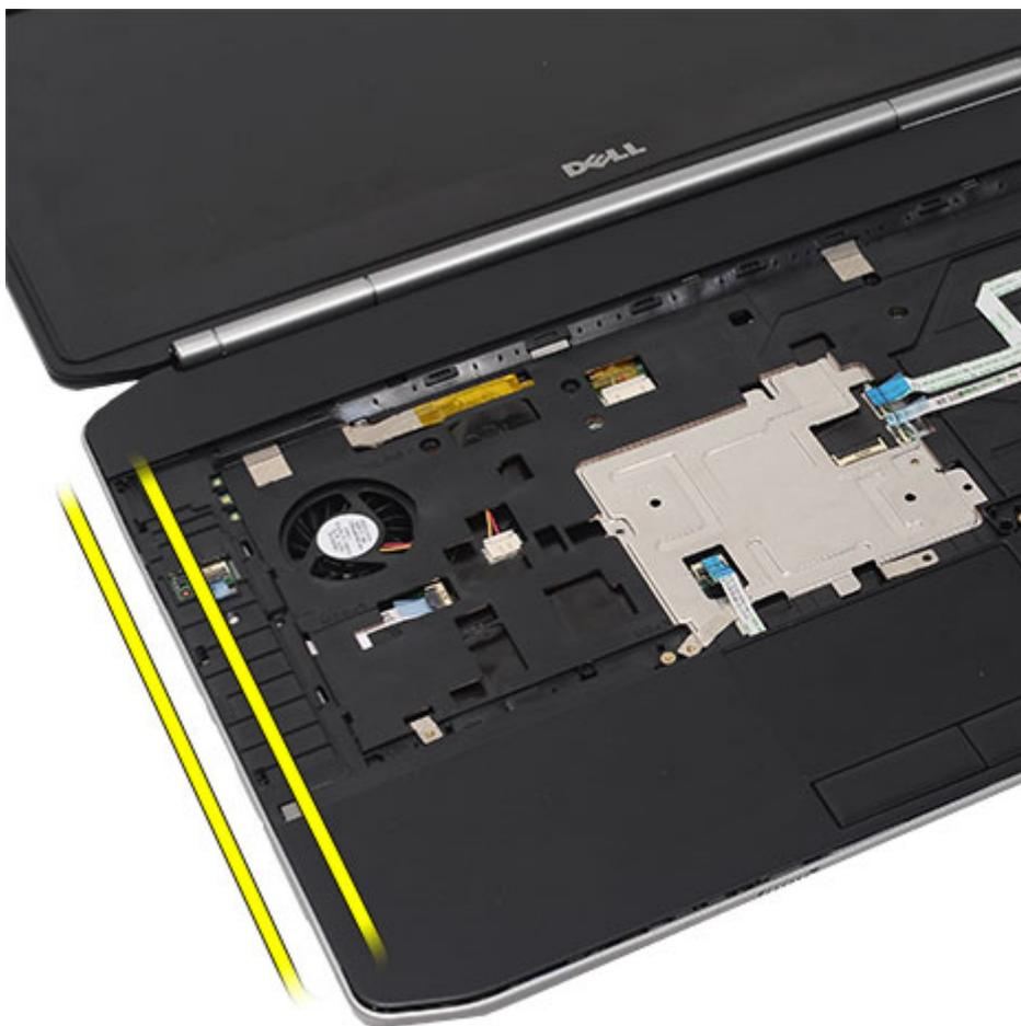
12. Release the tabs on the right edge of the palm rest assembly.
