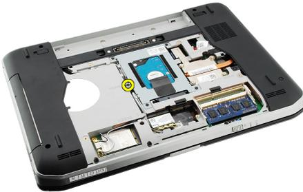
5. Push the screw tab away from the computer to release the optical drive from the drive bay.
