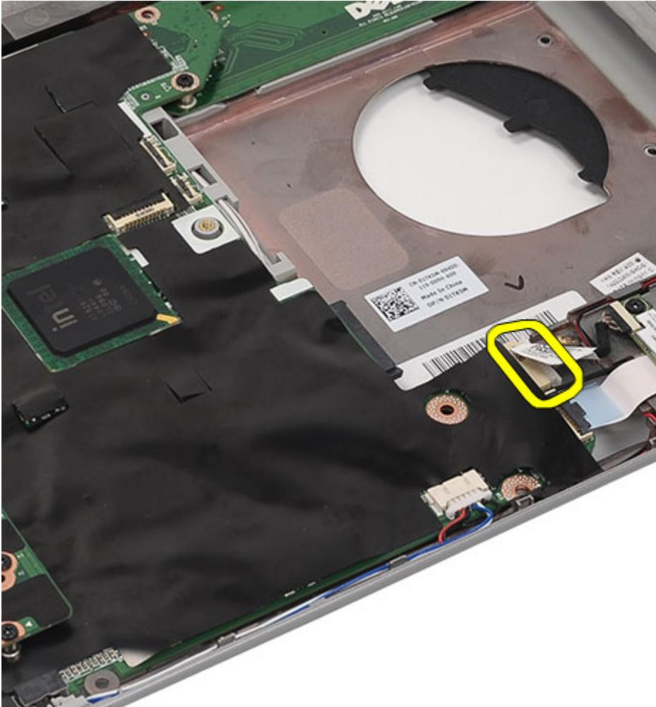
10. Remove the screw that secures the Bluetooth card.
