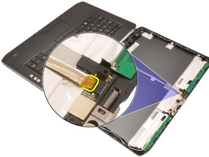
6. Loosen the screw that secures the camera module.
