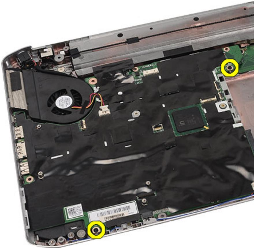
24. Lift the edge of the system board to disconnect it from the input/output (I/O) panel.
