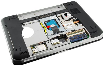
6. Remove the optical drive from the computer.
