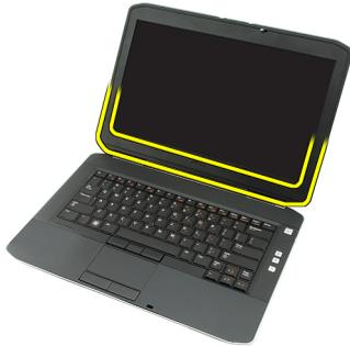
4. Work your way around the sides and the top edge of the display bezel.
