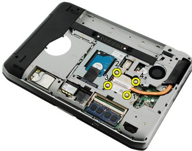
6. Lift the heat sink and remove it from the computer.
