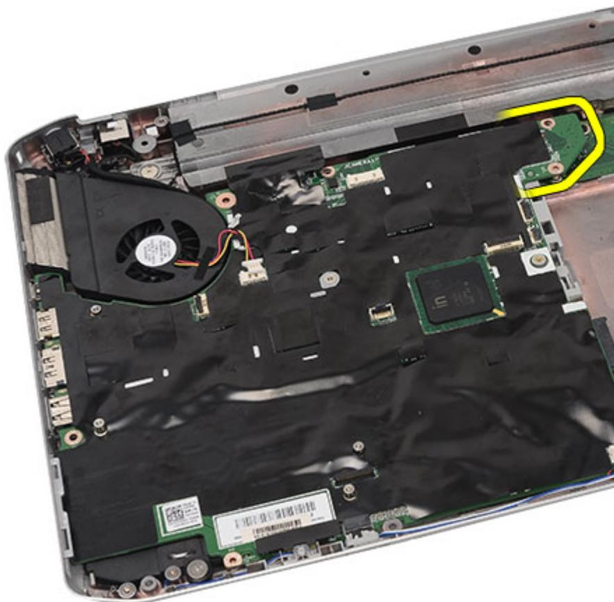
25. Release the system board from the port connectors.
