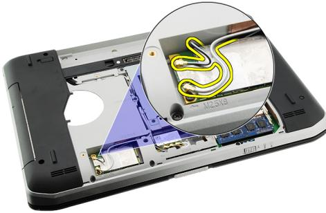
5. Remove the screw that secures the WWAN card to the system board.
