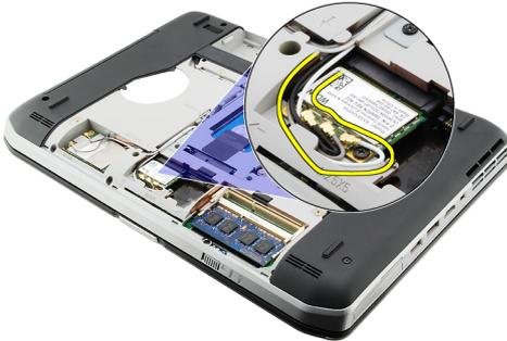
5. Remove the screw that secures the WLAN card to system board.
