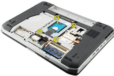
5. Use the tab to pull the hard-drive bracket upward and remove it from the computer.
