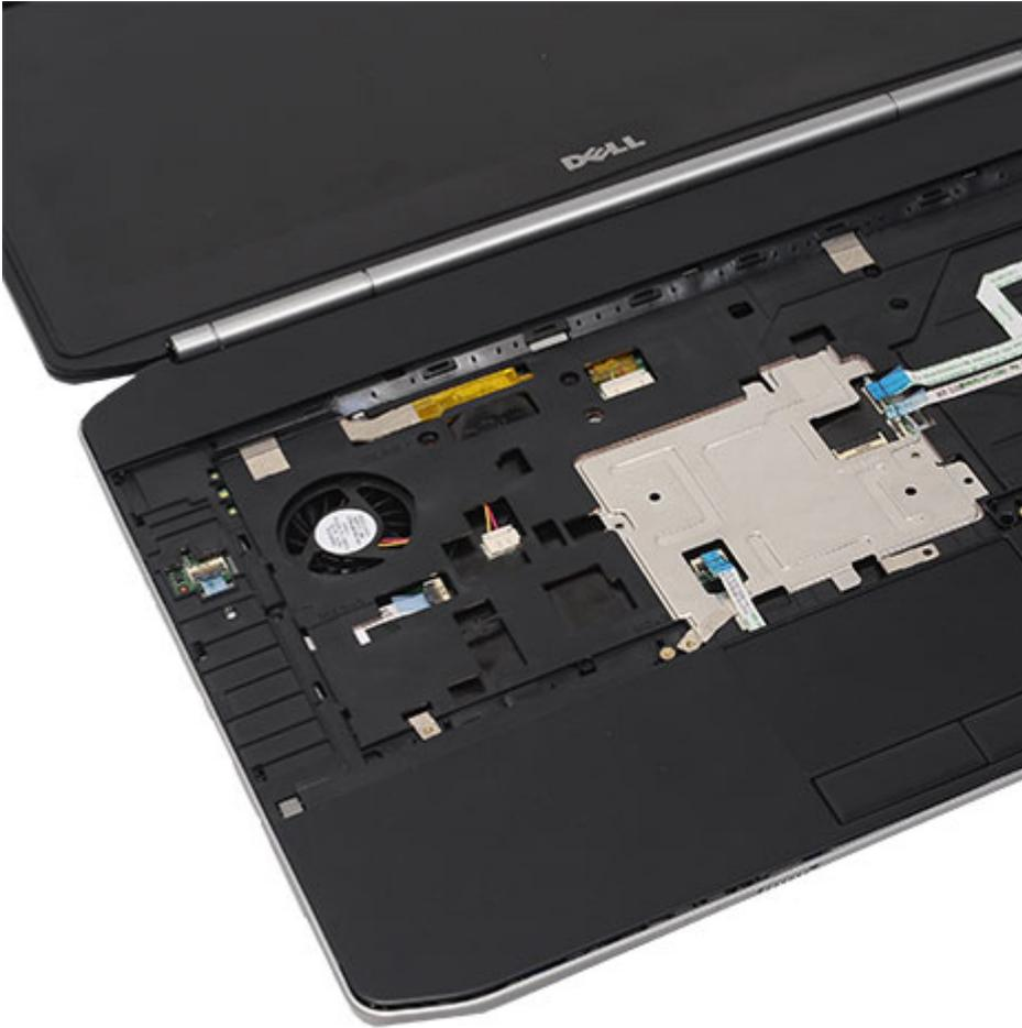
13. Remove the palm rest assembly from the computer.
