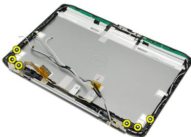
13. Remove the display hinges from the display assembly.
