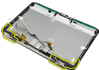
14. Separate the display hinge towers from the hinges.
