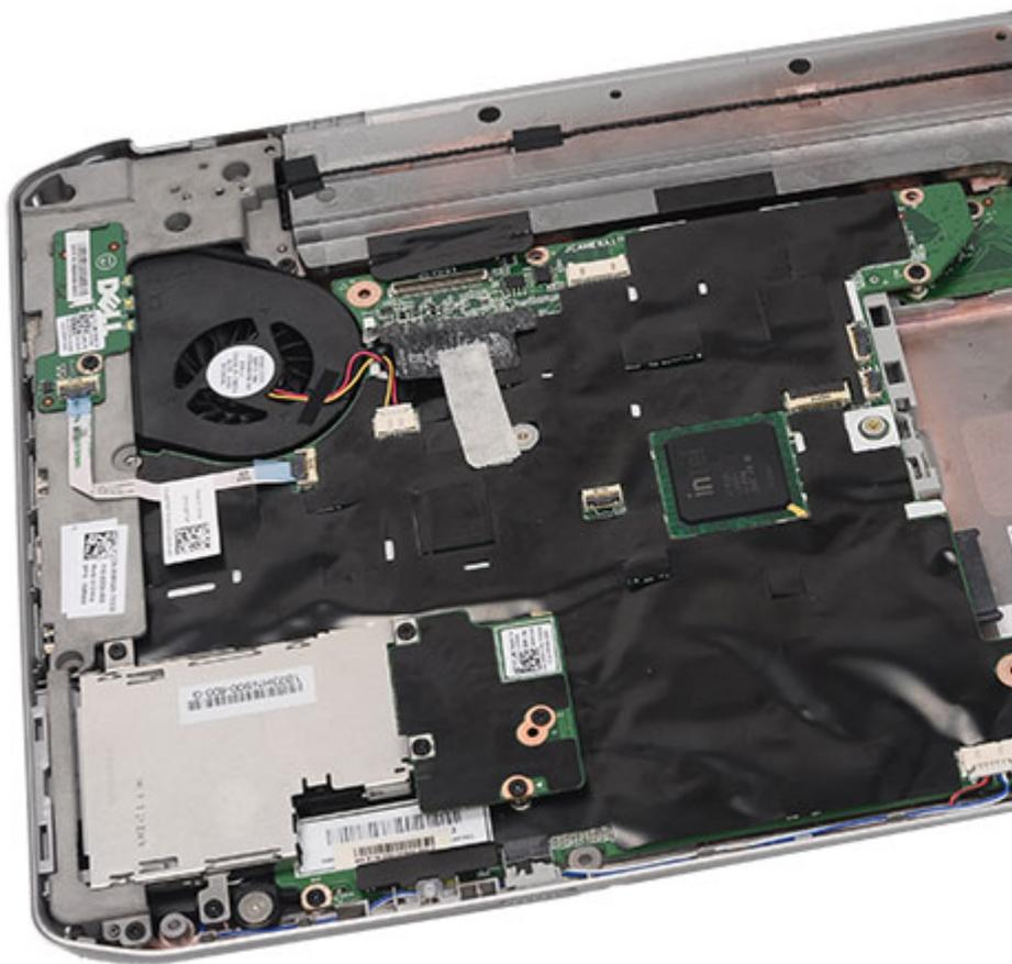
12. Remove the screws that secure the left support bracket.
