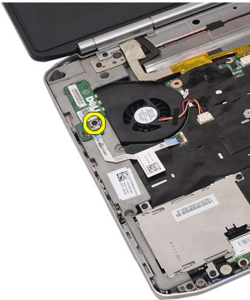
10. Disconnect the LED board cable from the system board connector.
