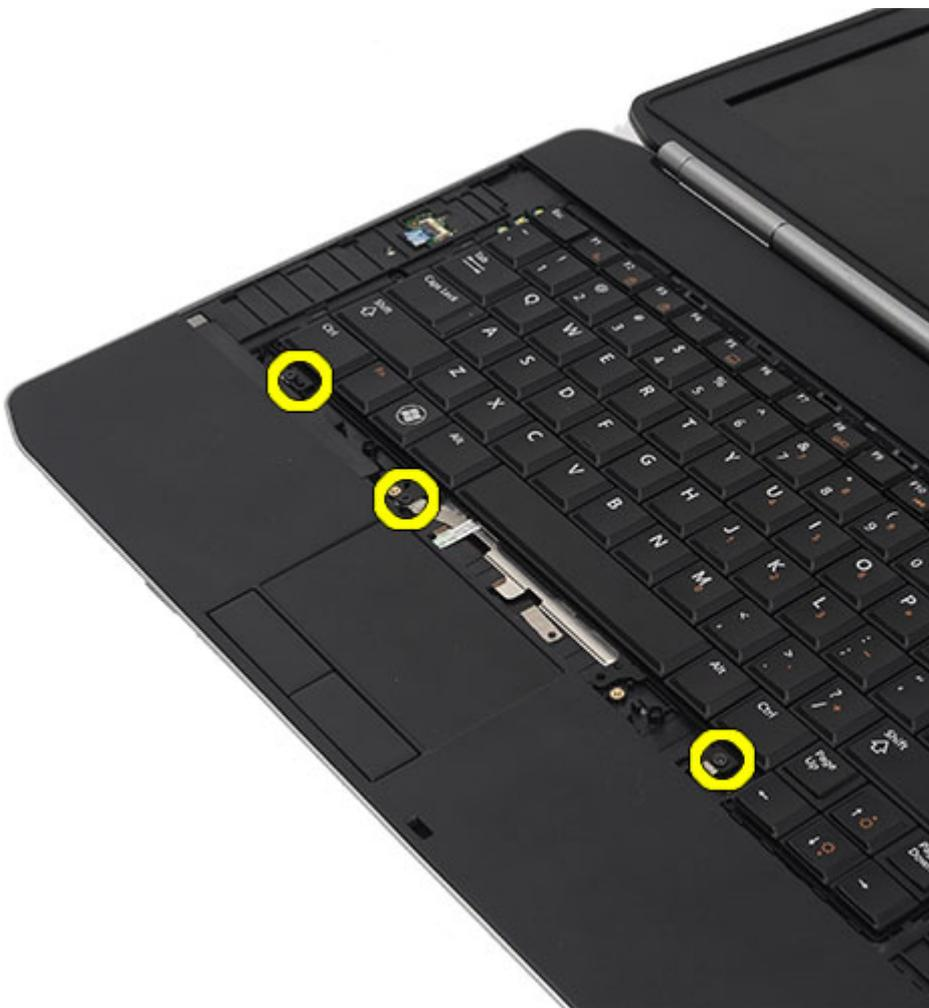
5. Flip the computer and remove the screws that secure the keyboard to the computer.
