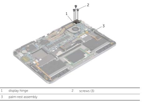
**3** Open the palm-rest assembly to release the display hinge and close the palm-rest assembly.
