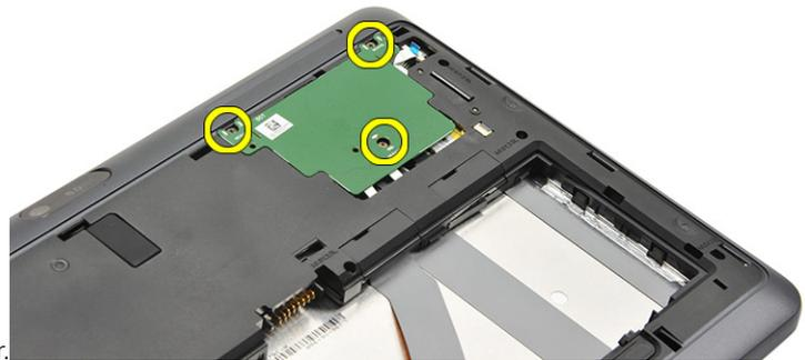
2. Remove the screws securing the SmartCard reader.
