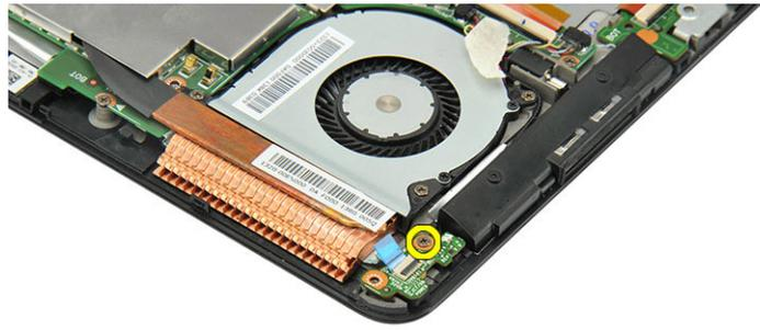
3. Remove the screw from the power switch board.
