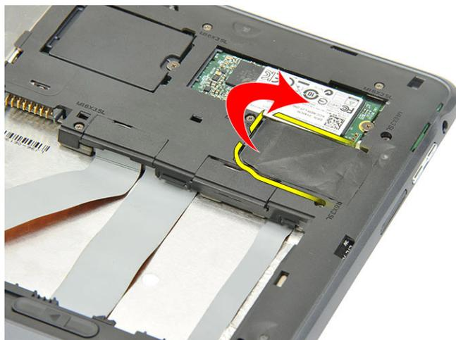
2. Tear off the mylar tape covering the WLAN card.
