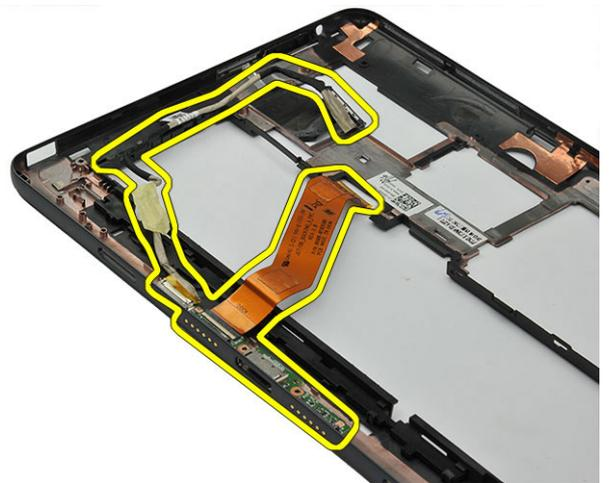
4. Lift to remove the docking board from the bottom case.
