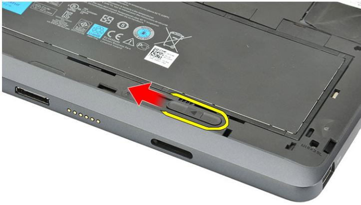
3. Remove the battery. Lift the battery away from the computer
