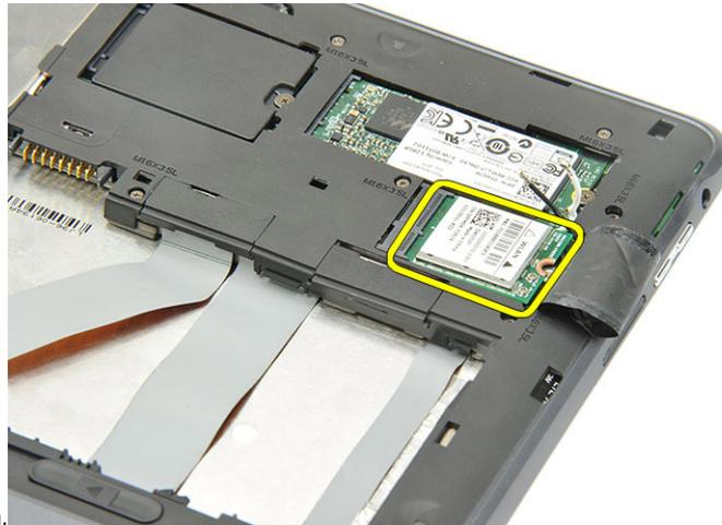
5. Remove the WLAN card from the system.
