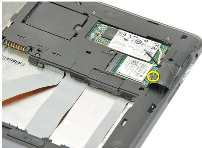
4. Remove the screw from the WLAN card.
