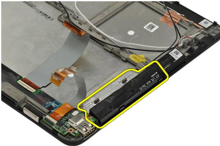
3. Remove the adhesive tapes on the speaker cables and remove the speaker module from the system.
