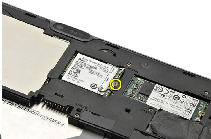
3. Remove the screw from the WWAN card.
