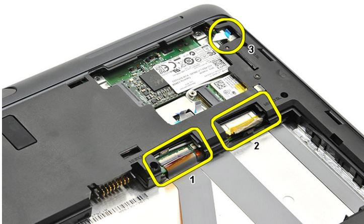
4. Pull up the docking FPC from the back of the LCD panel.
