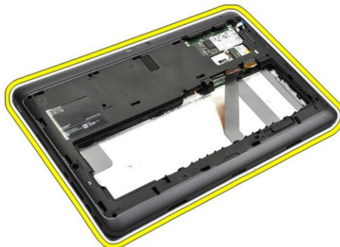
7. From the back of the bottom case, peel off the cables on top of the fingerprint reader.
