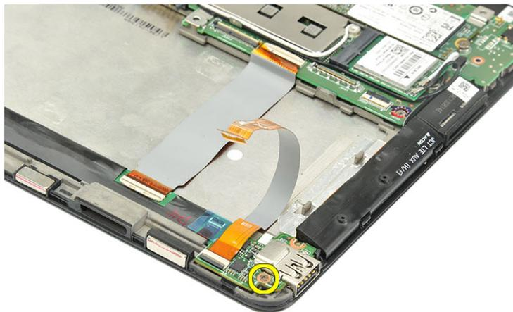
3. Remove the screw securing the USB board.
