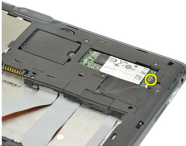
2. Remove the screw from the SSD.
