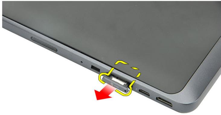
3. Slide the micro SD card cap out of the system.
