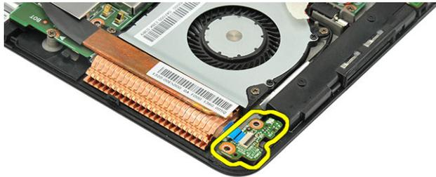
4. Remove the power switch board.
