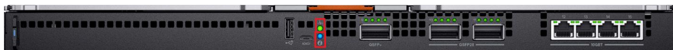
Figure 2a – Typical Fab A/B IO Module: Power/Status LED on the top and Identification LED on bottom as shown by red highlights.
