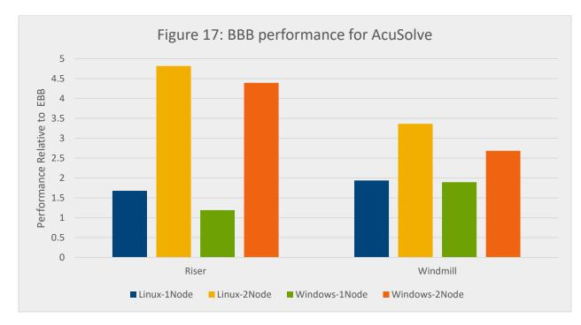
Here, the two node results for the Riser benchmark are artificially high, due to the effect of being able to fit this model into cache on two BBB's, but not into the reference 14G EBB server. This effect can be seen as well for the parallel speedup of this model on a system of EBB in Figure 4. Like Radioss, the BBB shows excellent overall performance both with Windows and with Linux. Again, the Linux based couplet offers a noticeable performance benefit over its Windows counterpart.
