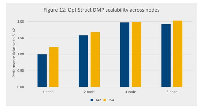
The reference for the plots was the single node 6142 server, where higher is better. One principle advantage of running OptiStruct jobs across nodes is that more memory and disk space is available when using multiple nodes, allowing larger models to be solved than could be solved using a single node. The results indicate good performance scalability when using multiple nodes.
