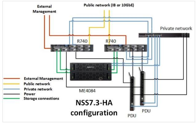
Figure 2 NSS7.3-HA Storage System Architecture
