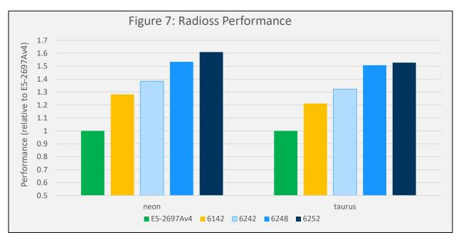
Here the performance is measured based on the elapsed solver time with the reference of 1.0 for the Dell EMC 13G Dell EMC R630 with dual Intel Xeon E5-2697Av4 16-core processors. The results are similar to the AcuSolve results, where the increase in performance from the 13G to the 14G servers is significant, particularly when 62xx series processors with a lot of cores are used.
