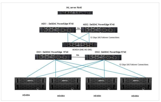
Figure 3 Dell EMC Ready Solution for Lustre Storage Reference Architecture
