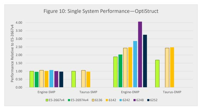
These results are shown relative to the performance of the 13G 8-core Intel Xeon E5-2667v4 based server, where higher indicates better overall performance. The E5-2667v4 based server had 512GB of memory with 2TB of local storage, the E5-2697Av4 server had 128GB of memory and 1TB of local storage, the 6136-based server had 384GB of memory and 2TB of disk space, and the remaining servers had 192GB of memory with 1TB of local storage.
