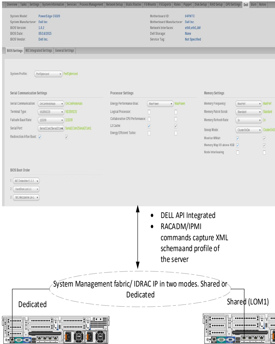
Figure 1. BIOS-level integration between Dell PowerEdge servers and Bright Cluster Manager 7.1.
