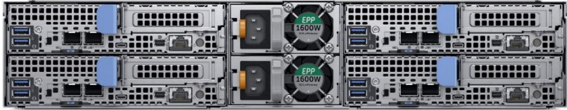
Figure 11 - PowerEdge C6400 chassis with four PowerEdge C6420 server sleds (rear view)
