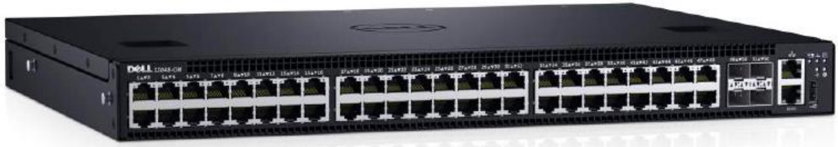
Figure 2 Dell Networking S3048-ON switch
