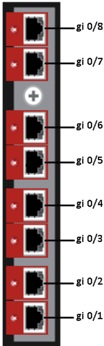
Figure 3. VRTX IOM switch module external port listing
