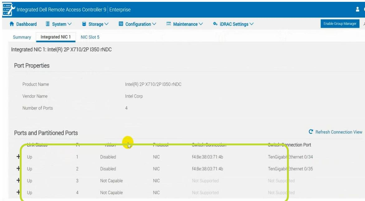
Figure 3 Viewing network device's Connection View information
