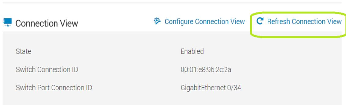
Figure 6 Refreshing iDRAC Connection View status
