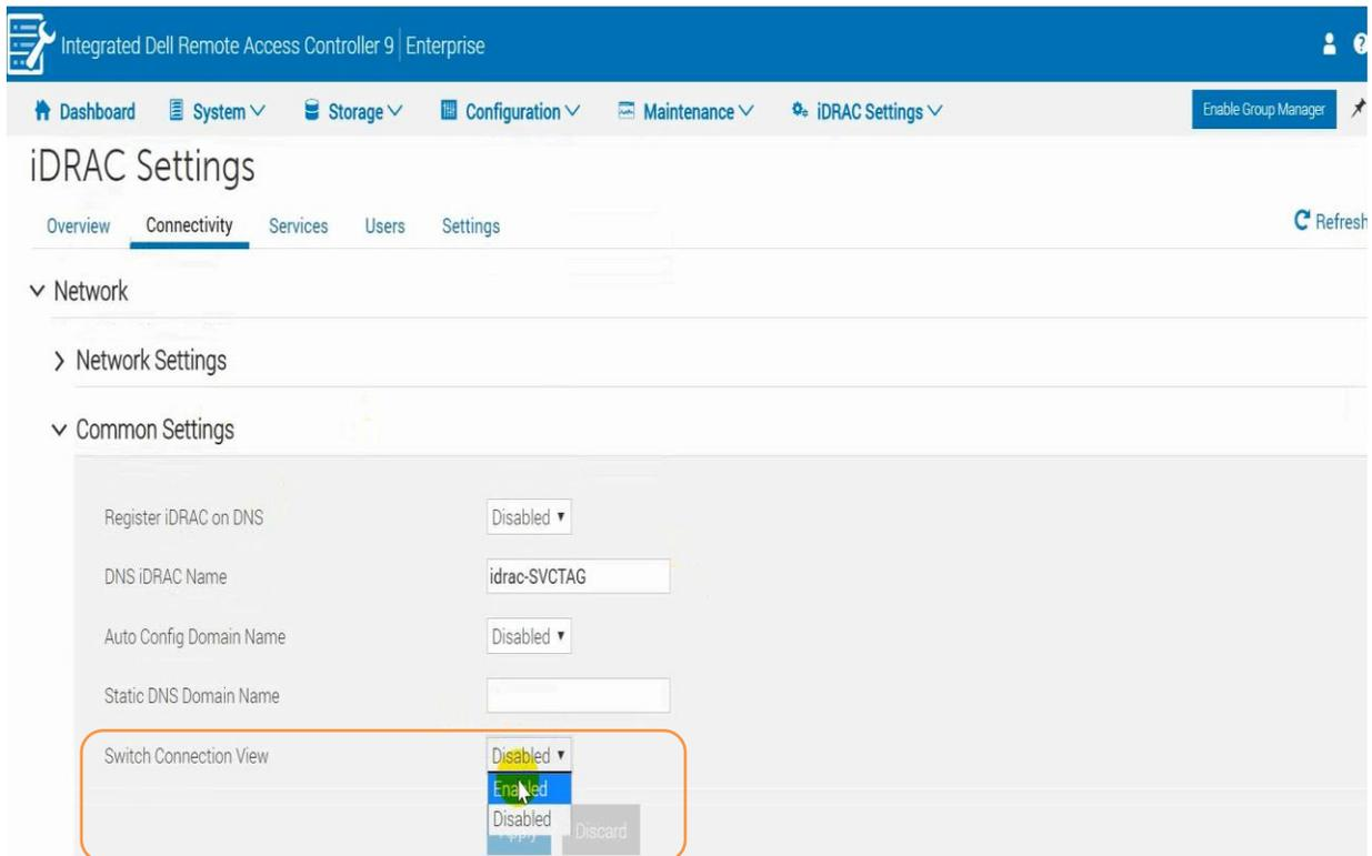
Figure 1 Enabling Switch Connection View by using iDRAC GUI
