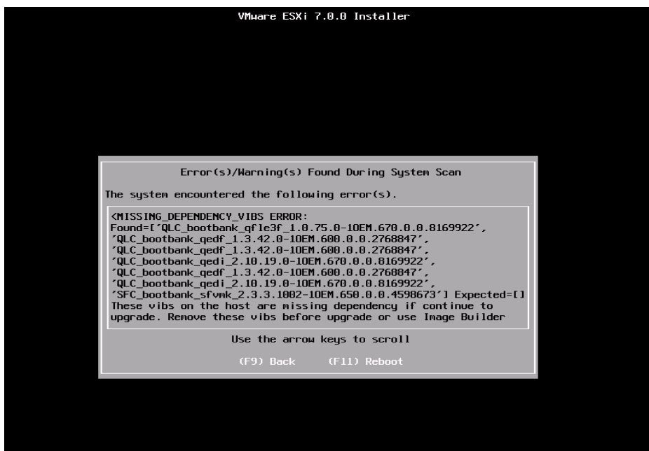
Figure 4 Upgrade failure from 6.7.x to 7.0 using ISO/CD Method
