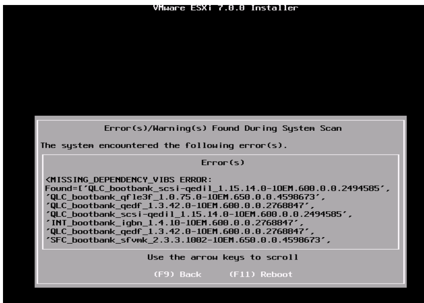
Figure 1 Upgrade failure from 6.5.x to 7.0 using ISO/CD
