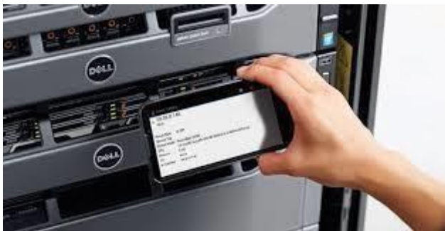
Figure 1 An administrator using iDRAC Quick Sync
