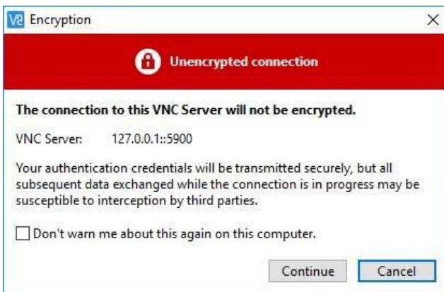
Figure 15 Unencrypted connection to the VNC server
