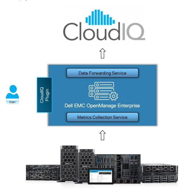
Figure 1 Metrics collected from iDRAC and forwarded to CloudIQ via OME
