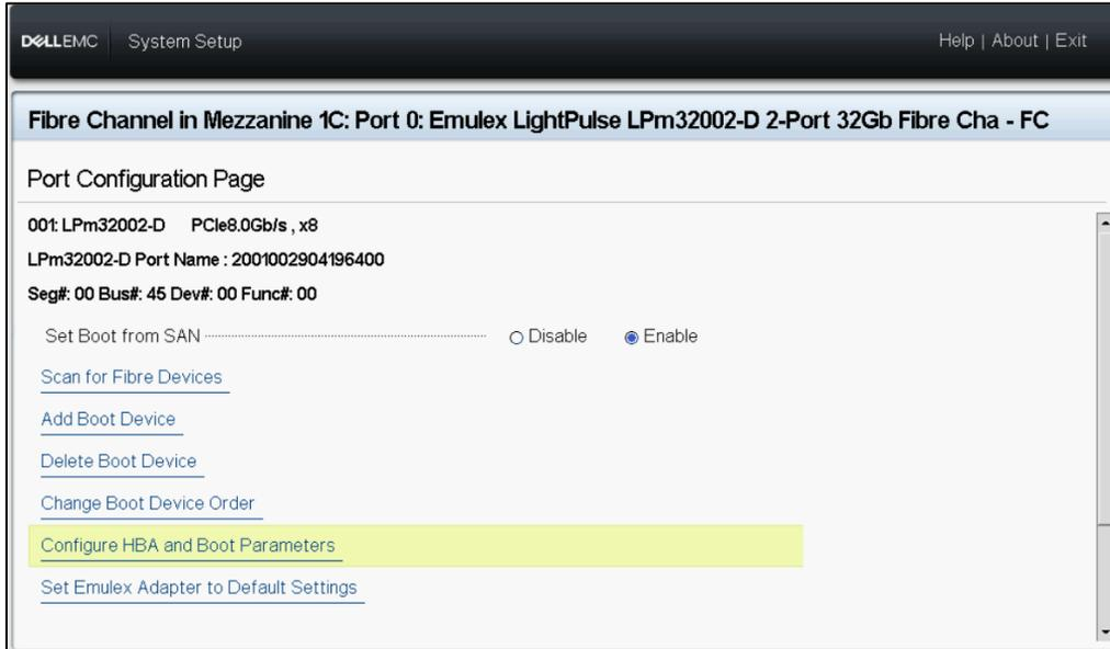
2. Once the FC Target parameters are provided, the base system is now available for connection with the Storage Target LUN. However, this configuration uses the physical identities hardwired to the FC card, the data is prone to loss in case of failure.
