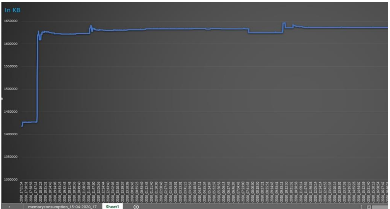
Figure 2 Task Execution Service Memory utilization (in KB) while testing the firmware upgrade feature for 200 servers of Dell EMC OpenManage Enterprise 3.4 on PowerEdge servers
