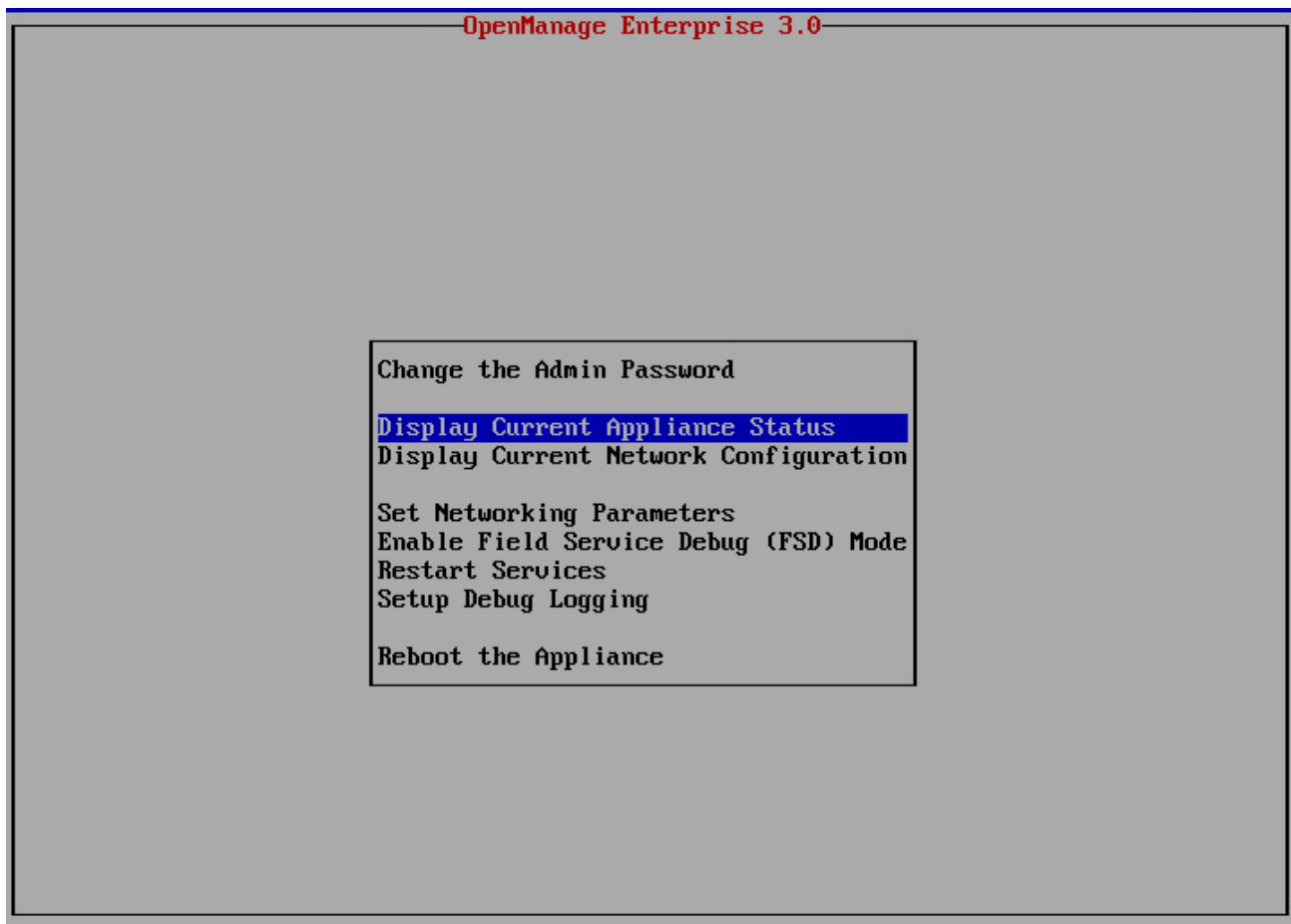
Figure 15 View current network status of OpenManage Enterprise
