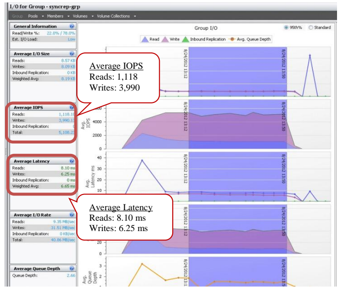
Figure 13: SANHQ metrics for 3 PS6100X at 4500 user load with SyncRep enabled during switchover operation
