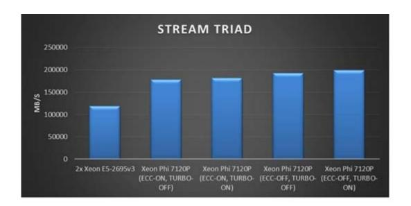
The achieved stream bandwidth on CPU only configuration on R730 was taken as the baseline. We observe performance improvements of 50% to 70% on configurations with one Intel Xeon® Phi 7120P and two Intel Xeon® Phi 7120P as against the CPU only configuration. The best STREAM bandwidth was observed on Intel Xeon® Phi 7120P with ECC set to OFF and turbo set to ON.
