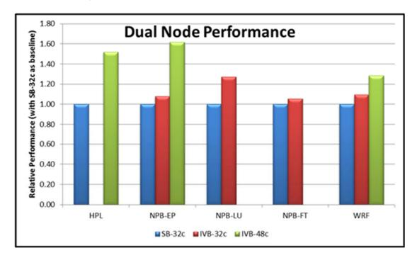
HPL was executed on a two node cluster with E5-2665 (total 32 cores, 16 cores per server) and E5-2695 v2 (total 48 cores, 24 cores per server). HPL yielded 1.52x sustained performance on IVB-48c as compared to SB-32c whereas WRF, NPB-EP and NPB-LU have shown a performance improvement of ~2.5%. There is ~7 %- 8% increase in the performance with WRF and NPB-EP on 32 cores. It is ~ 22 – 32% difference when compared between 48 cores E5-2695 v2 and 32 cores E5-2665 runs.
