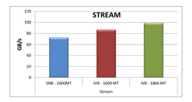
The graph compares the memory bandwidth of the E5-2600 v2 processor to its predecessor, the E5-2600. With E5-2600, the maximum supported memory speed is 1600MT/s. With E5-2600 v2, that maximum is 1866MT/s. We've compared 1600MT/s DIMMs for SB-16c and IVB-24c, and also plotted the improved memory bandwidth with 1866MT/s on IVB-24c.
