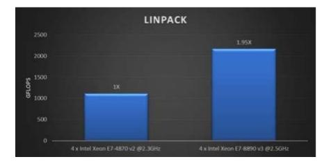
As shown in the graph above, LINPACK showed 1.95X performance improvement with four Intel Xeon E7-8890 v3 processors on R930 server in comparison to four Intel Xeon E7-4870 v2 processors on R920 server. This was due to substantial increase in number of cores, memory speed, flop/second of the processor and processor architecture.
