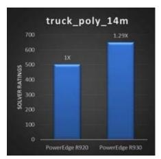
We used four different datasets for Fluent. We considered 'Solver rating' (higher is better) as the performance metric. For all the test cases with PowerEdge R930 Fluent showed 24% to 29% performance improvement in-comparision to PowerEdge R920.
