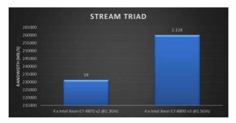
This chart showed the comparison of sustained memory bandwidth between PowerEdge R920 and PowerEdge R930 servers. STREAM showed 231GB/s on PowerEdge R920 and 260GB/s on PowerEdge R930, which is 12% improvement in memory bandwidth. This increase is because of the improvement in DIMM speed available on PowerEdge R930.
