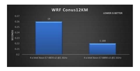
With Conus12KM dataset, WRF showed 0.22seconds average time on PowerEdge R930 server, while 0.26seconds on PowerEdge R930 server, which is an 18% improvement.
