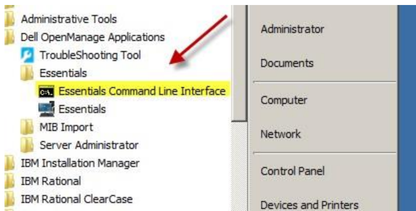
Figure 1 CLI Access Point
